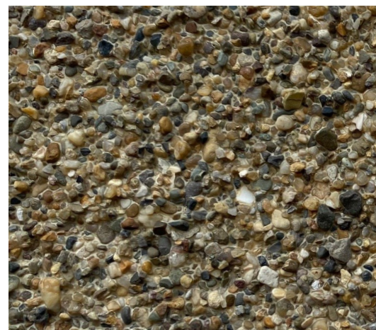
▲ Reference material for darker resin surface treatment for pedestrian lanes and heavy trafficked public spaces
