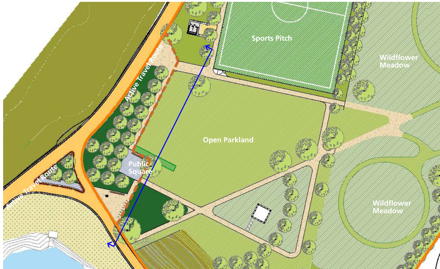
▲ Proposed Plan of Stop Point C and intersection of Active Travel and leisure route to the east. Currently, the ATR proposals incorporate the western corridor of proposed 'Port Park' which is delineated as a 'share with care' surface for pedestrians and cyclists
