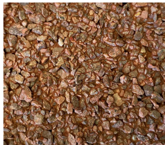
▲ Reference material for a reddish coloured surface treatment incorporated for ATR cycle lanes along the route
