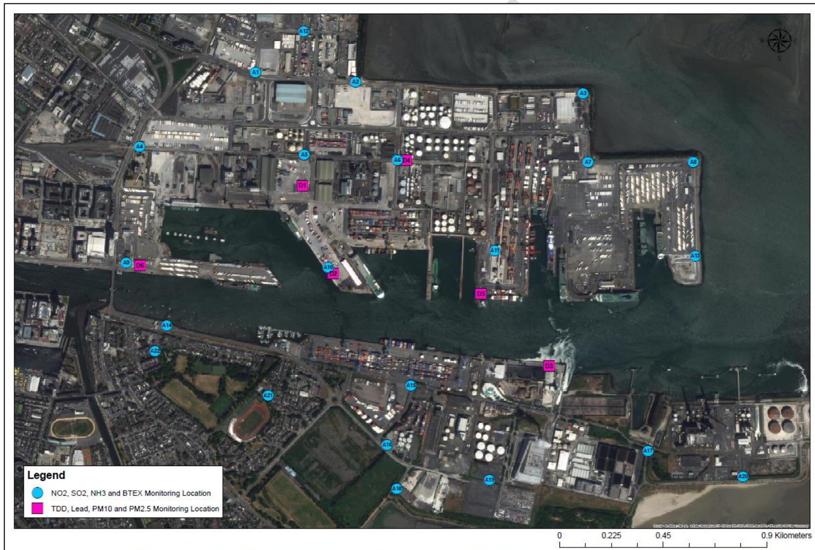
Figure 10.48: Overview of Ambient Air Monitoring Locations Located Within Dublin Port and Surrounding Environs for Nitrogen Dioxide, Sulphur Dioxide, BTEX, Ammonia, Total Depositional Dust, PM 10/2.5 and Lead
