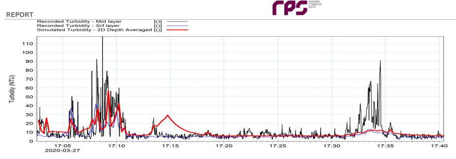
Figure 8.42: Comparison of recorded and simulated turbidity measurements across the dump site during Event 374
