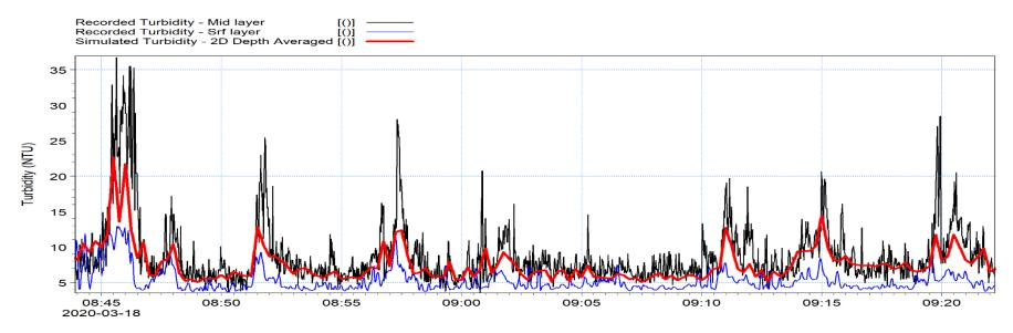
Figure 8.37: Comparison of recorded and simulated turbidity measurements across the dump site during Event 280
