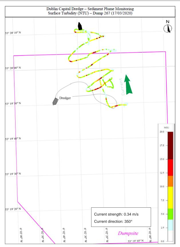
Figure 8.5: Dump 267 Survey track with surface turbidity [NTU]
