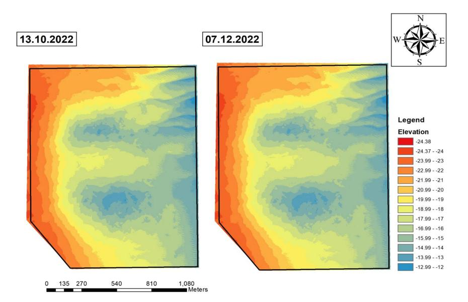
Figure 4-14 Pre and post dredging campaign bathymetric surveys at the licenced offshore dump site at the approaches to Dublin Bay
