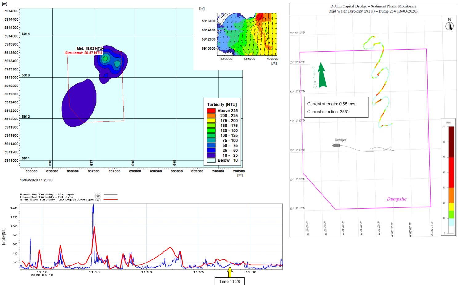
Figure 6.2 Event 254. 2D Sediment plume envelope c. 21min after initial sediment release with current speed and direction insert (top left). Extent of survey data (top right) and comparison with simulated data (bottom left)
