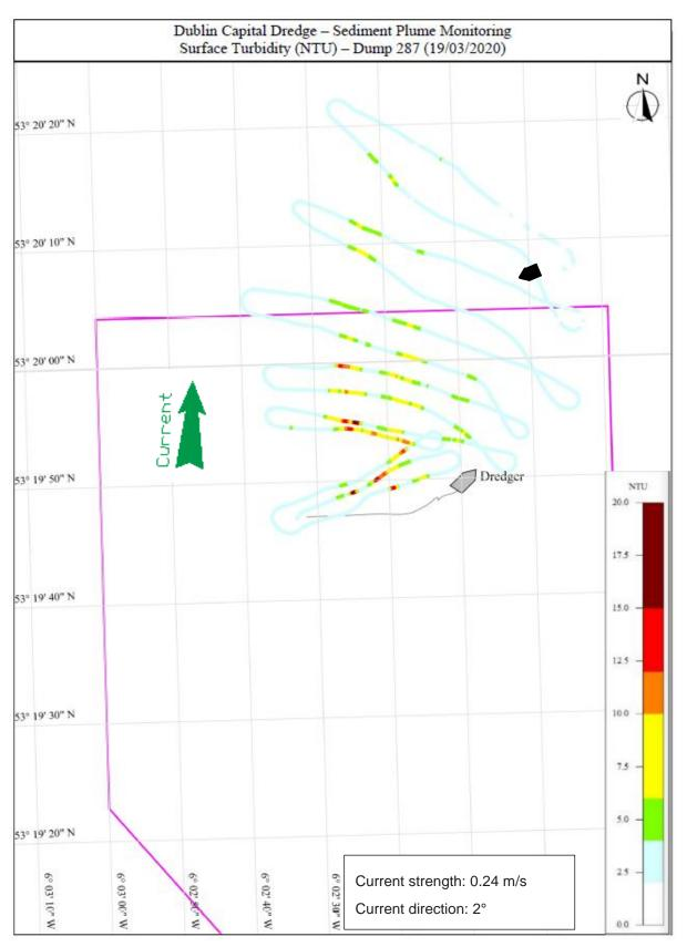
Figure 8.21: Dump 287 Survey track with surface turbidity [NTU]
