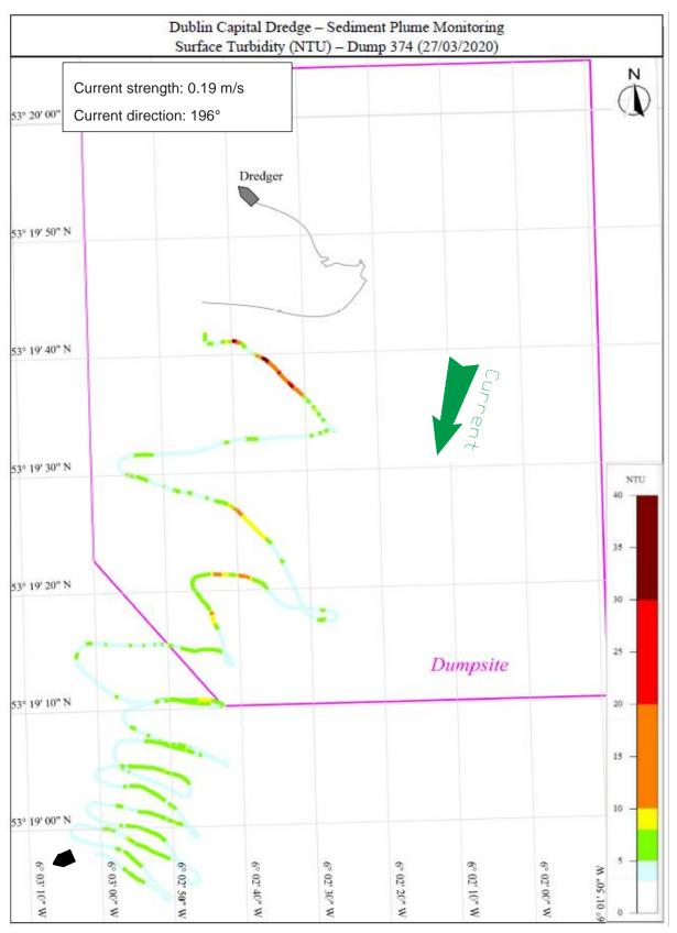
Figure 8.28: Dump 374 Survey track with surface turbidity [NTU]
