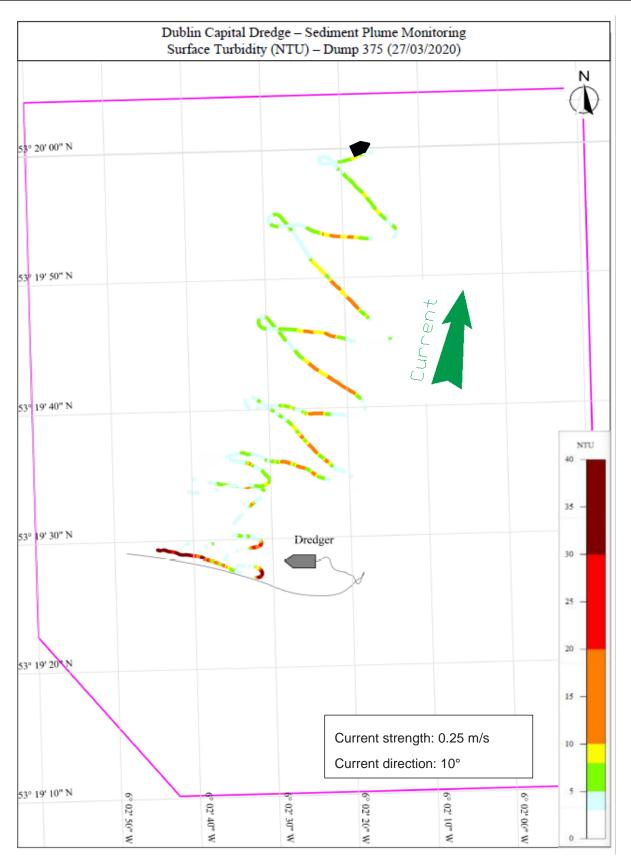
Figure 8.30: Dump 375 Survey track with surface turbidity [NTU]
