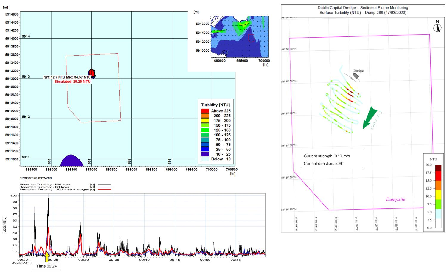
Figure 6.3 Event 266. 2D Sediment plume envelope c. 6min after initial sediment release with current speed and direction insert (top left). Extent of survey data (top right) and comparison with simulated data (bottom left)
