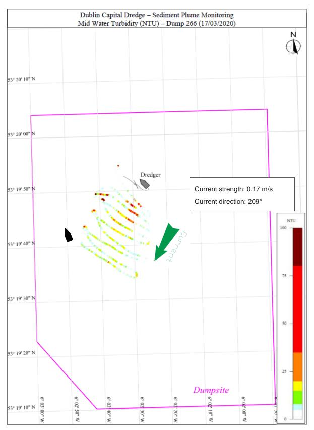
Figure 8.4: Dump 266 Survey track with mid water turbidity [NTU]
