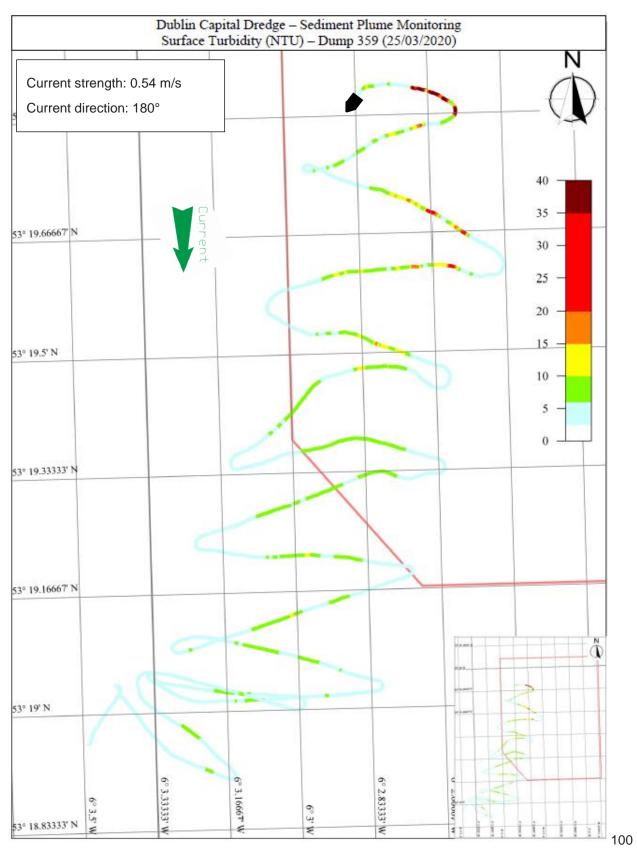
Figure 8.25: Dump 359 Survey track with surface turbidity [NTU]
