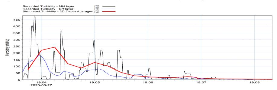
Figure 8.43: Comparison of recorded and simulated turbidity measurements across the dump site during Event 375
