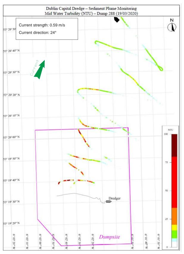
Figure 8.24: Dump 288 Survey track with mid water turbidity [NTU]
