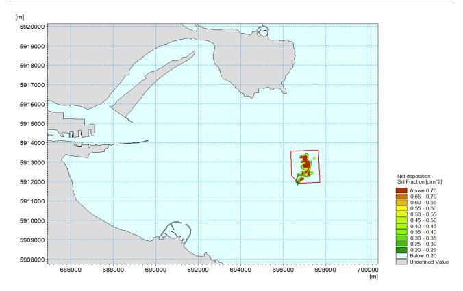
Figure 4-6 Total deposition of silt material following the dumping at sea activities associated with the MP2 Project (S0024-02)
