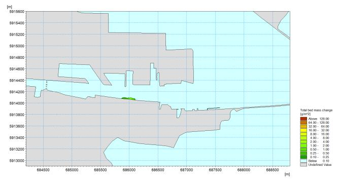
Figure 3-2 3FM Project - Deposition of sediment following dredging activity at South Port Berths for a proposed Ro-Ro Terminal (Localised Scour Protection to 220 kV cables)
