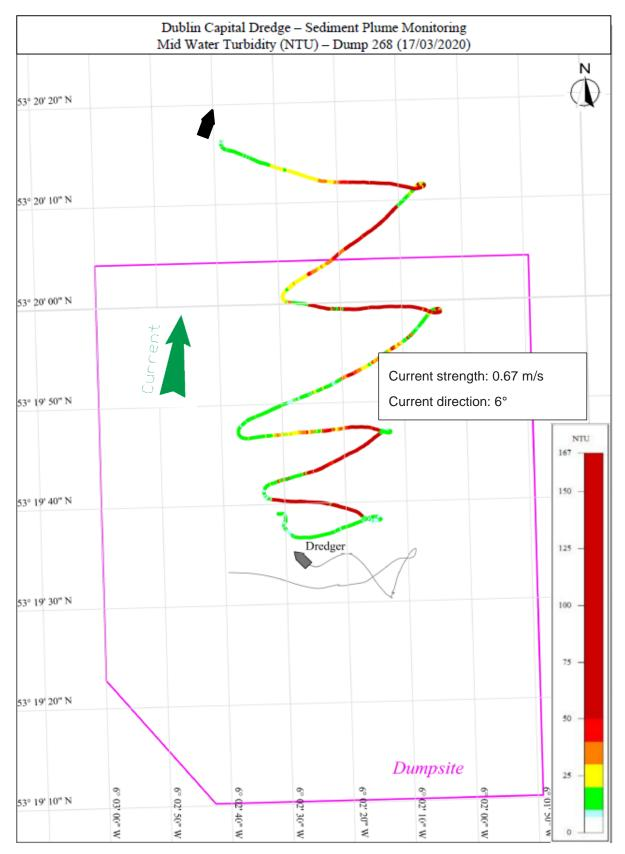
Figure 8.8: Dump 268 Survey track with mid water turbidity [NTU]
