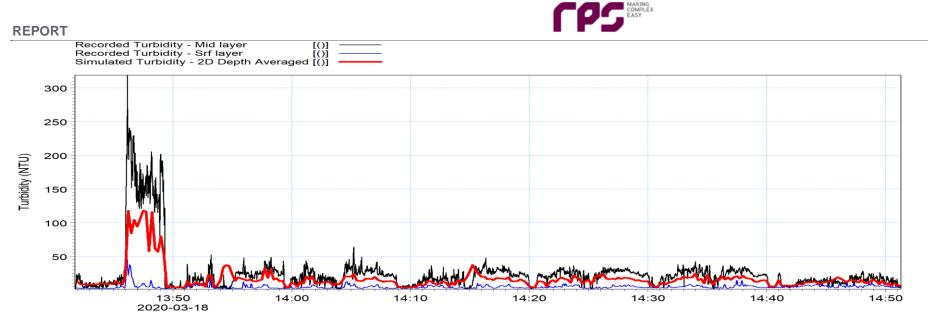
Figure 8.40: Comparison of recorded and simulated turbidity measurements across the dump site during Event 283
