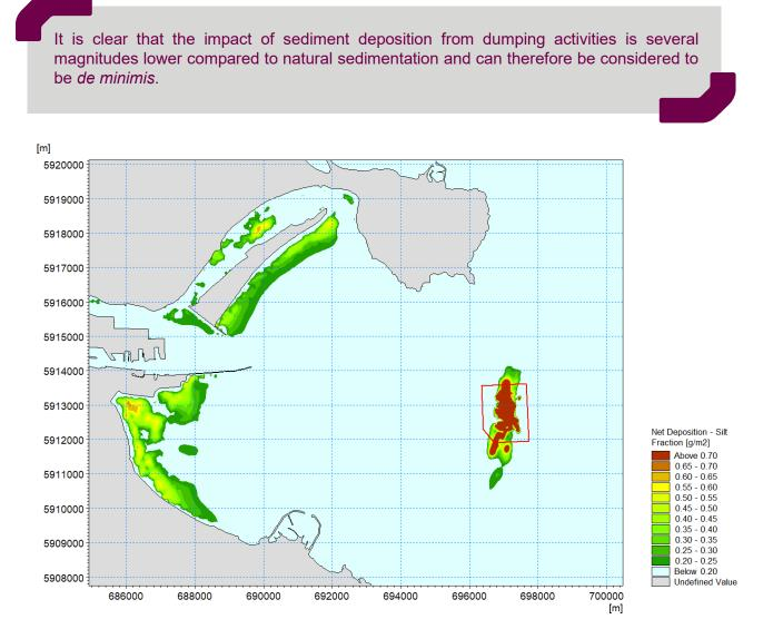
Figure 4-10 Cumulative total deposition of silt material following the dumping at sea activities associated with S0024-02, S0004-03, S0033-01 and the 3FM Project
