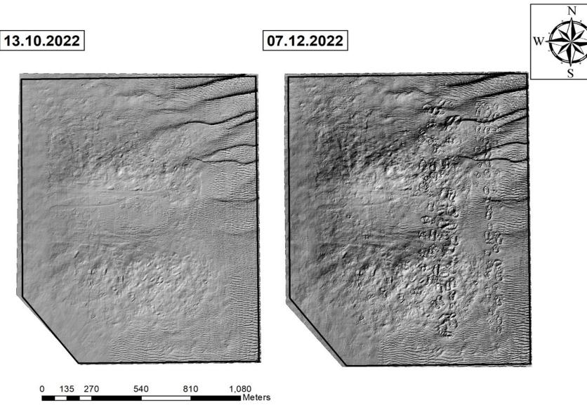
Figure 4-15 Sand wave and other morphological features identified from a terrain analyses of both survey datasets
