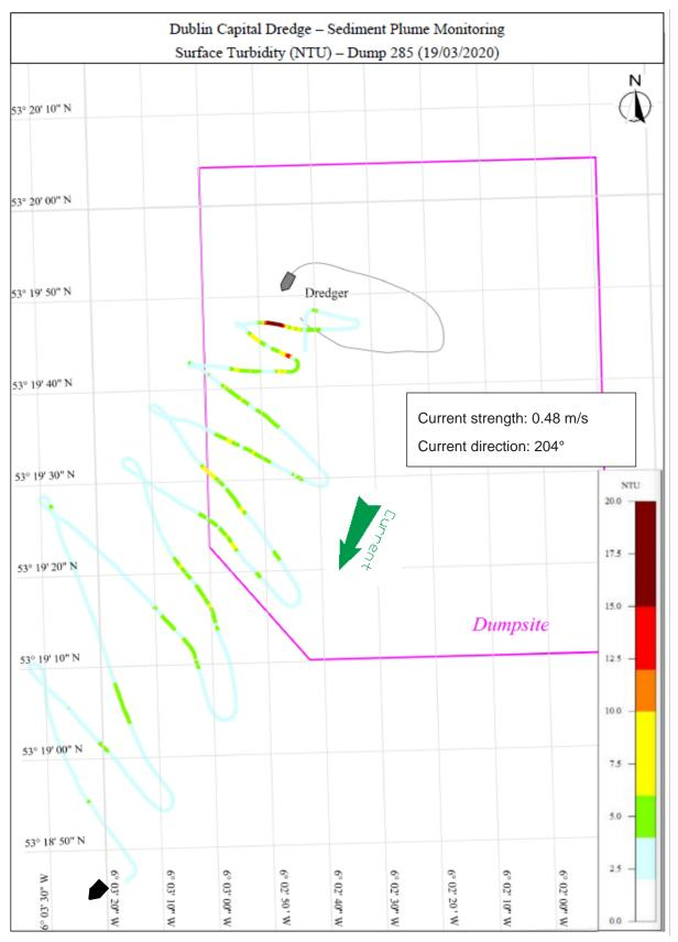
Figure 8.18: Dump 285 Survey track with surface turbidity [NTU]
