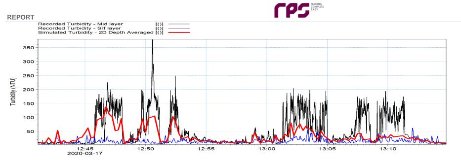
Figure 8.36: Comparison of recorded and simulated turbidity measurements across the dump site during Event 268
