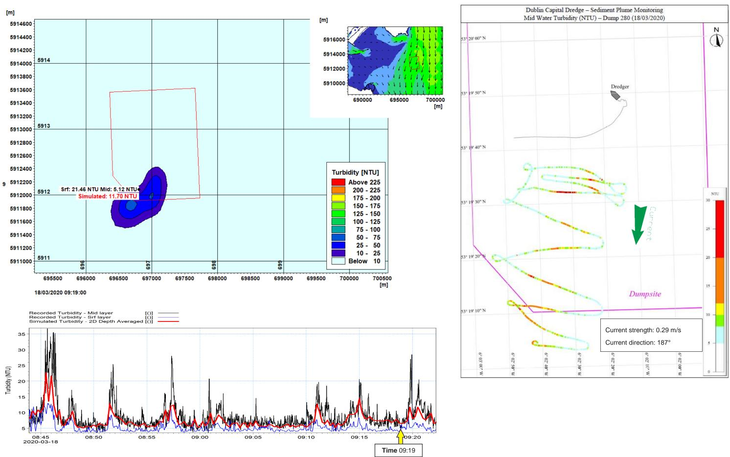
Figure 6.6 Event 280. 2D Sediment plume envelope c. 28min after initial sediment release with current speed and direction insert (top left). Extent of survey data (top right) and comparison with simulated data (bottom left)
