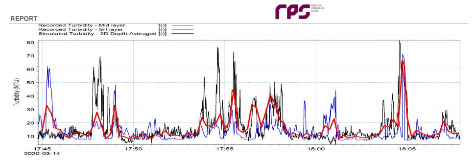
Figure 8.32: Comparison of recorded and simulated turbidity measurements across the dump site during Event 231
