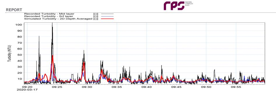
Figure 8.34: Comparison of recorded and simulated turbidity measurements across the dump site during Event 266
