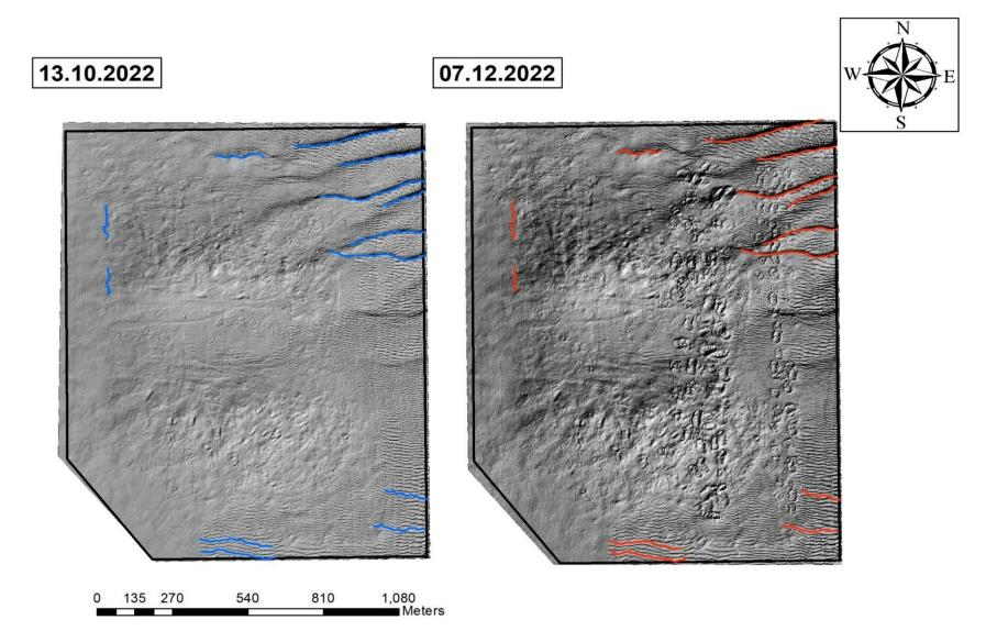
Figure 4-16 Sand wave features common to both surveys identified by blue and red vectors that were used to assess movement of bed material
