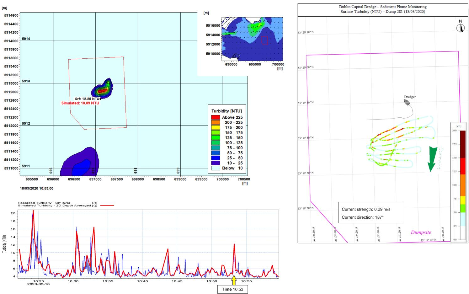
Figure 6.7 Event 281. 2D Sediment plume envelope c. 31min after initial sediment release with current speed and direction insert (top left). Extent of survey data (top right) and comparison with simulated data (bottom left)
