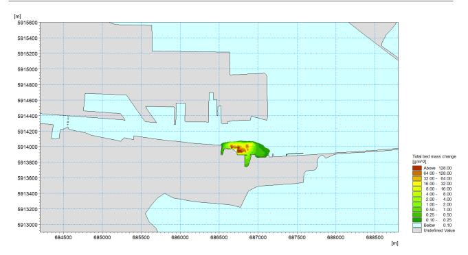
Figure 3-3 3FM Project - Deposition of sediment following capital dredging activity at the Sludge Jetty to create a proposed Turning Circle
