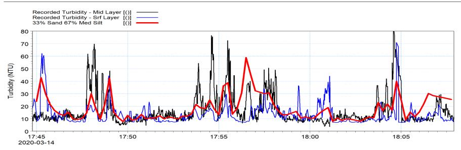
Figure 5.4: Comparison of recorded and simulated turbidity levels during dump event 231 – Mixture 3 (33% fine sand; 67% medium silt)
