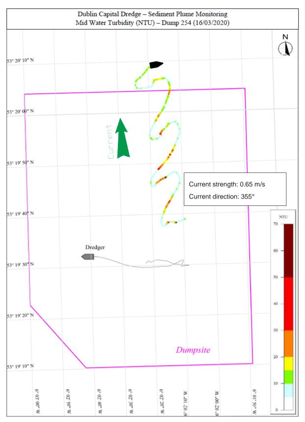
Figure 8.2: Dump 254 Survey track with mid water turbidity [NTU]
