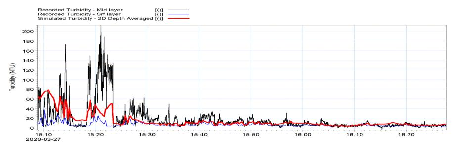
Figure 8.41: Comparison of recorded and simulated turbidity measurements across the dump site during Event 373
