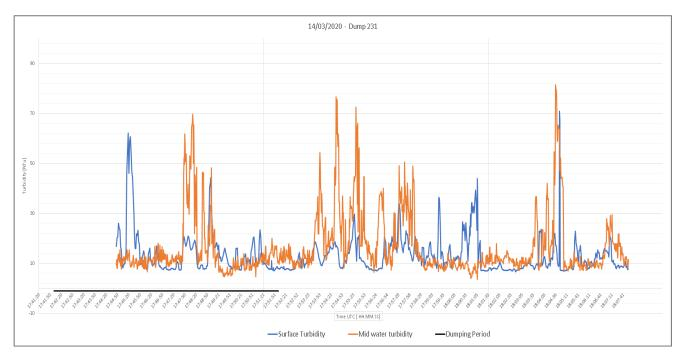
Figure 3.3: Example turbidity readings at the surface and mid-point of the water column during Dump Trip 231
