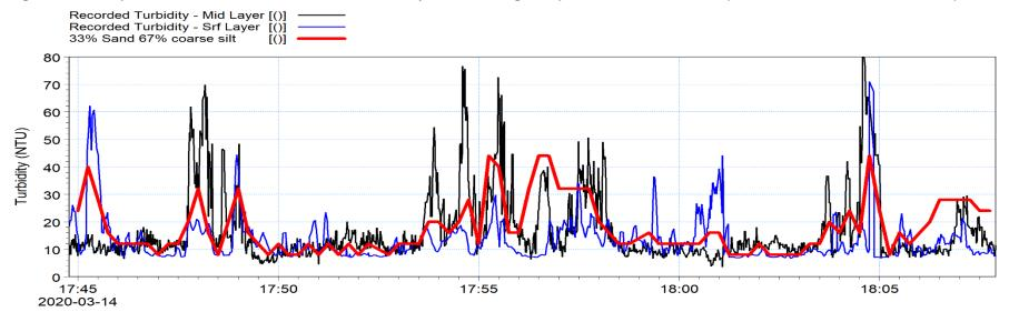
Figure 5.5: Comparison of recorded and simulated turbidity levels during dump event 231 – Mixture 4 (33% fine sand; 67% coarse silt)
