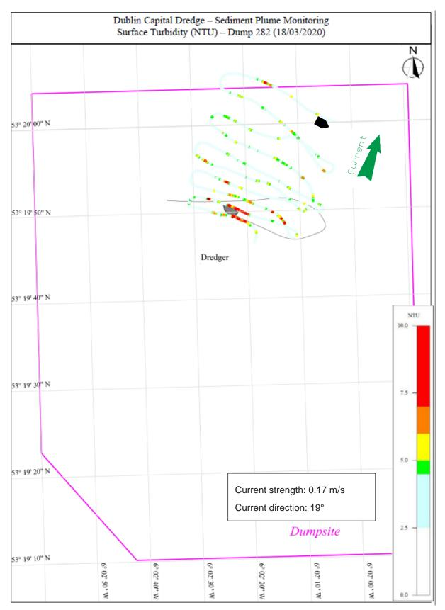
Figure 8.12: Dump 282 Survey track with surface turbidity [NTU]
