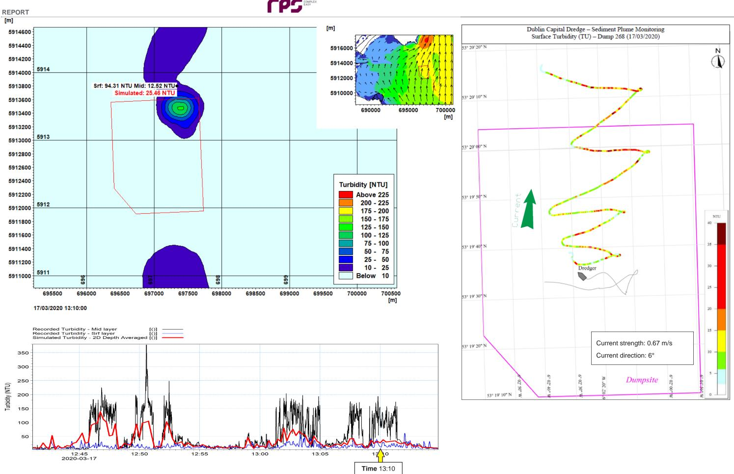
Figure 6.5 Event 268. 2D Sediment plume envelope c. 30min after initial sediment release with current speed and direction insert (top left). Extent of survey data (top right) and comparison with simulated data (bottom left)
