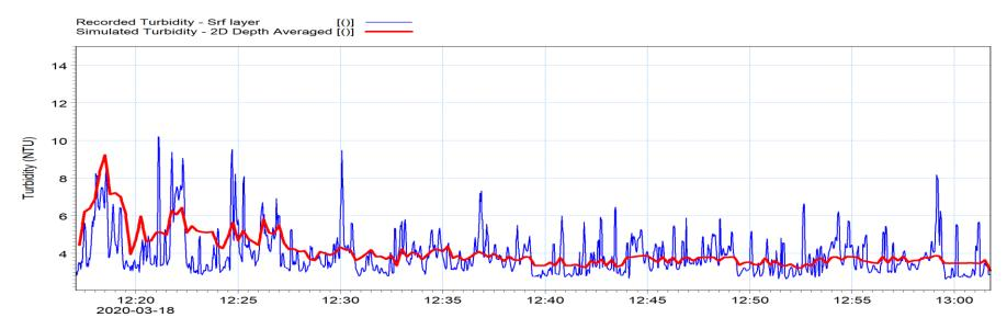
Figure 8.39: Comparison of recorded and simulated turbidity measurements across the dump site during Event 282
