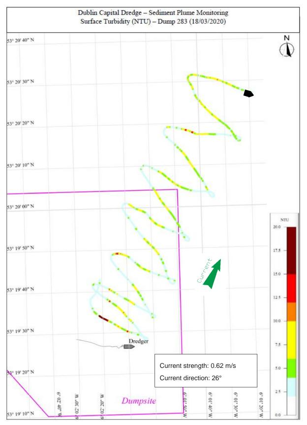
Figure 8.14: Dump 283 Survey track with surface turbidity [NTU]
