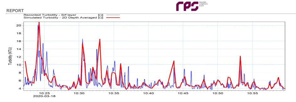
Figure 8.38: Comparison of recorded and simulated turbidity measurements across the dump site during Event 281
