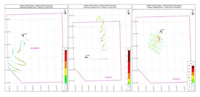
Figure 4-2 TSHD track during the disposal of sediment across three individual dumping activities (trips) with the corresponding measured suspended sediment concentration
