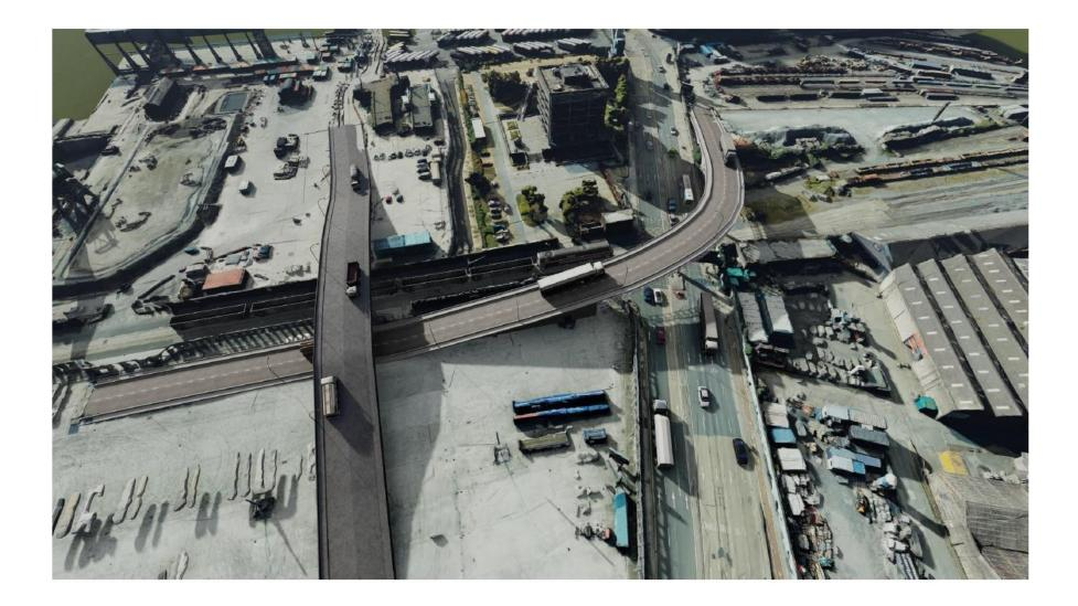
Appendix 6 : screen grabs of PARAMICS traffic model showing impact of two trains per hour crossing into the port via the at grade rail crossing of East Wall Road, and from there on to a rail intermodal at Alexandra Quay East
