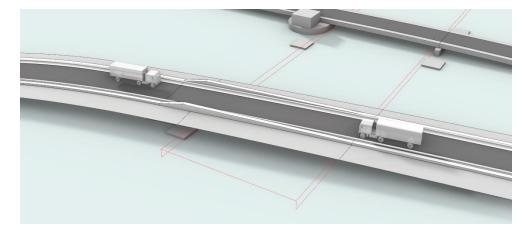
Figure 6: Option 2B: Rolling Bascule with the rolling mechanism and counterweight below deck level
