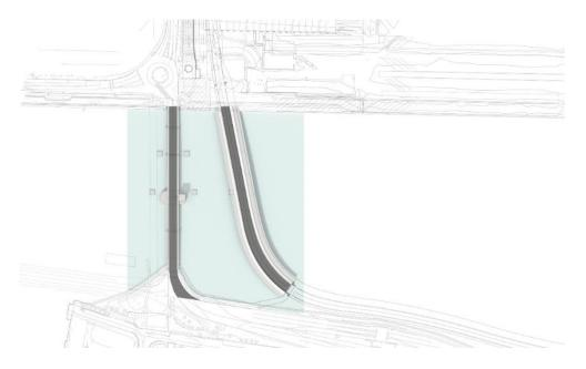
Figure 1: Existing Tom Clarke Bridge (left) with the proposed alignment for the new crossing (right)
