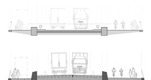
Figure 14: Design development of deck cross section
