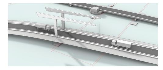
Figure 2: Option 1: Dutch Bascule
