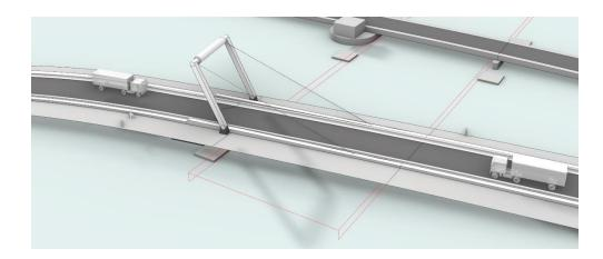
Figure 10: Option 4A: Double Pivoting Bascule with a counterweight supported above the deck
