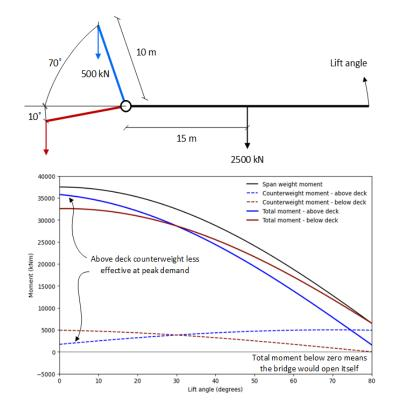
*Figure 13: Simplified example bascule arrangement with either an above-deck or below-deck counterweight, illustrating the effectiveness of each solution.*
