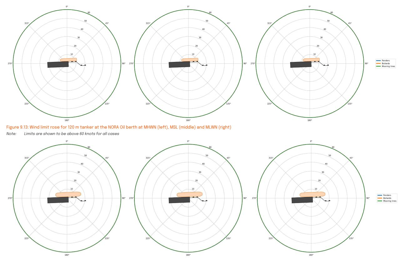
Figure 9.14: Wind limit rose for 185 m tanker at the NORA Oil berth at MHWN (left), MSL (middle) and MLWN (right) Note: Limits are shown to be above 60 knots for all cases
