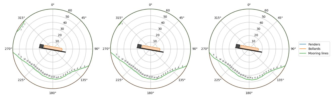
Figure 9.17: Wind limit rose for MV Celine at Berth 45 at MHWN (left), MSL (middle) and MLWN (right)
