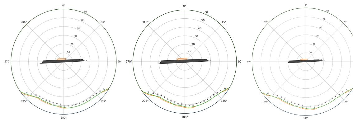
Figure 9.9: Wind limit rose for 150 m container ship at the New South Bank Container Terminal at MHWN (left), MSL (middle) and MLWN (right)
