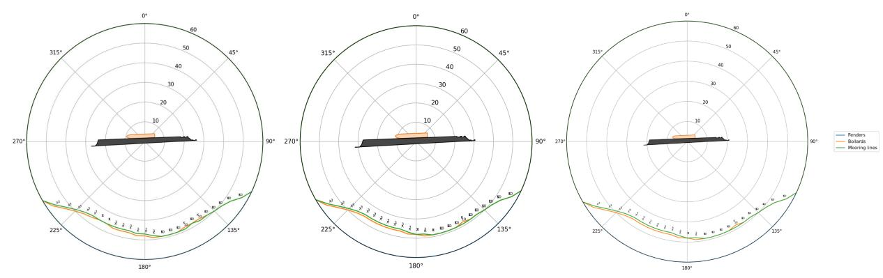
Figure 9.10: Wind limit rose for 225 m container ship at the New South Bank Container Terminal at MHWN (left), MSL (middle) and MLWN (right)
