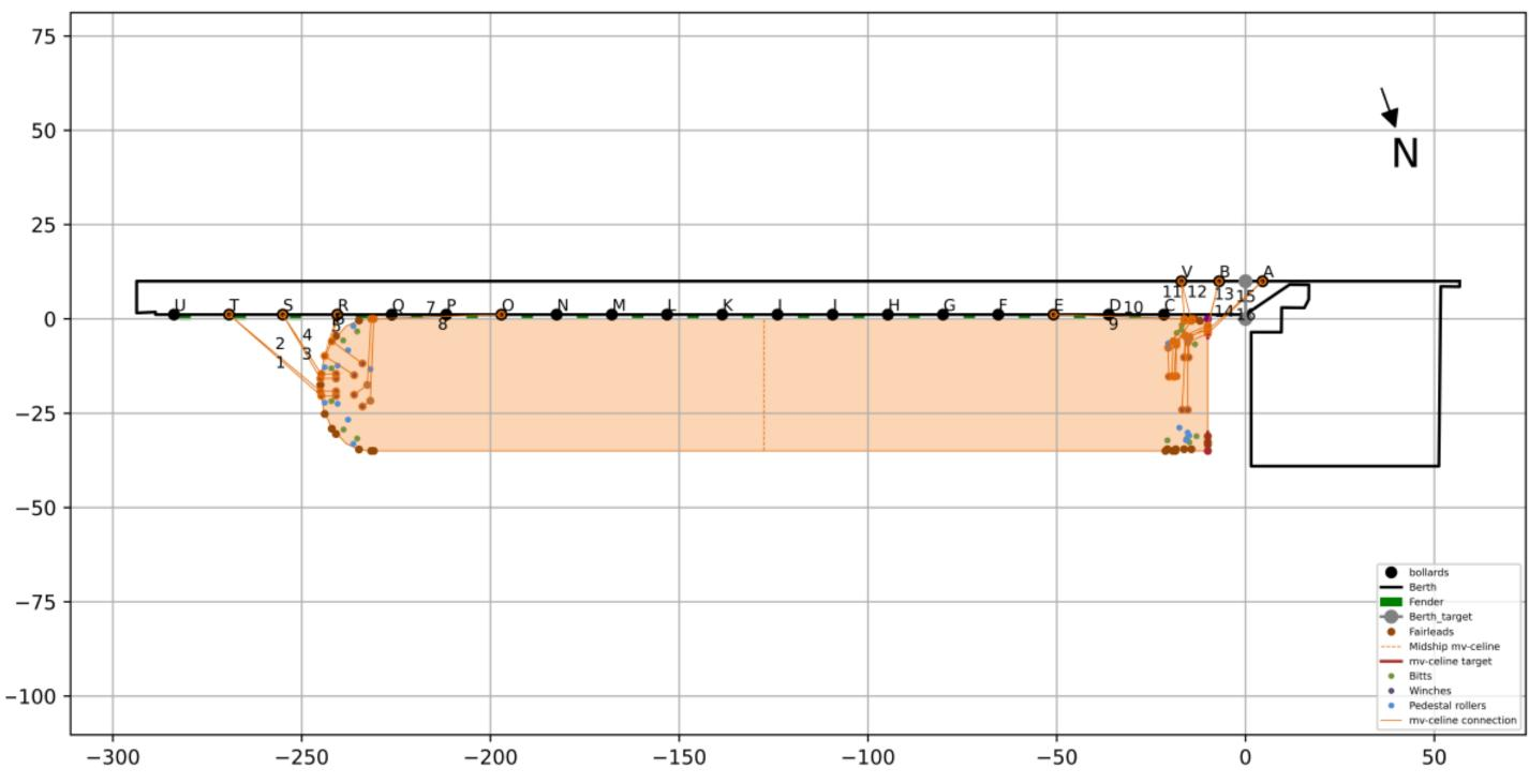
Figure 9.16: Mooring arrangement for MV Celine at Berth 45
