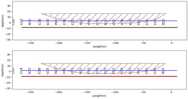
Figure 9.6: Fender contacts for MV Celine at MHWN (top) and MLWN (bottom)
