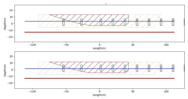
Figure 9.4: Fender contacts for 185 m tanker at MHWN (top) and MLWN (bottom)
