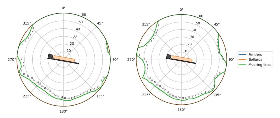
Figure 9.18: Wind limit rose for MV Celine at Berth 45 at MHWN for 20 m (left) and 30 m (right) setback bollards at the bow and stern
