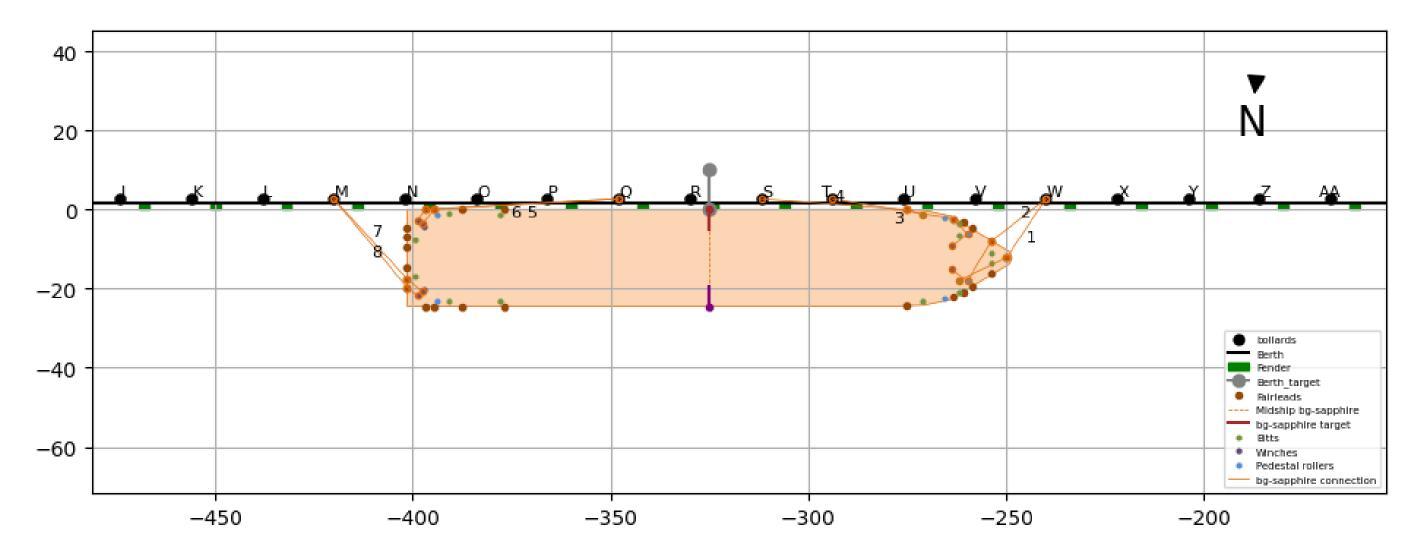
Figure 9.7: Mooring arrangement for 150 m container ship at the New South Bank Container Terminal
