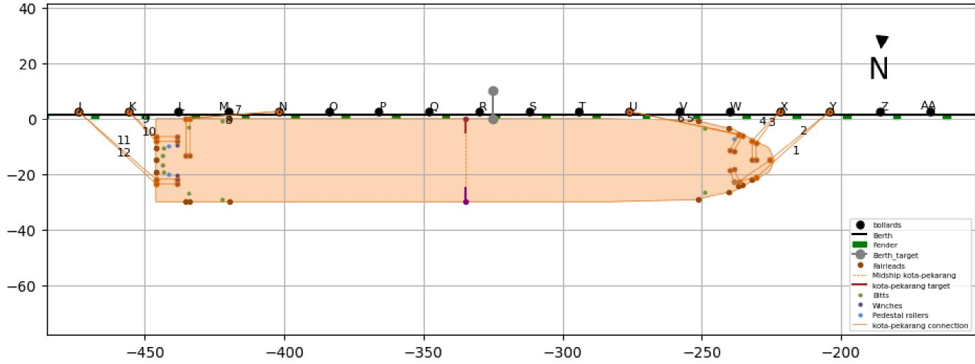
Figure 9.8: Mooring arrangement for 225 m container ship at the New South Bank Container Terminal
