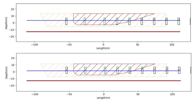
Figure 9.5: Fender contacts for 185 m tanker at MHWN (top) and MLWN (bottom)
