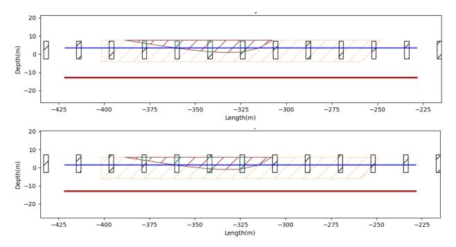
Figure 9.1: Fender contacts for 150 m container ship at MHWN (top) and MLWN (bottom)
