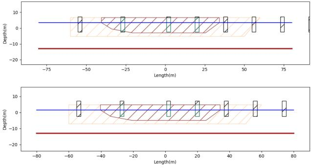
Figure 9.3: Fender contacts for 150 m container ship at MHWN (top) and MLWN (bottom)
