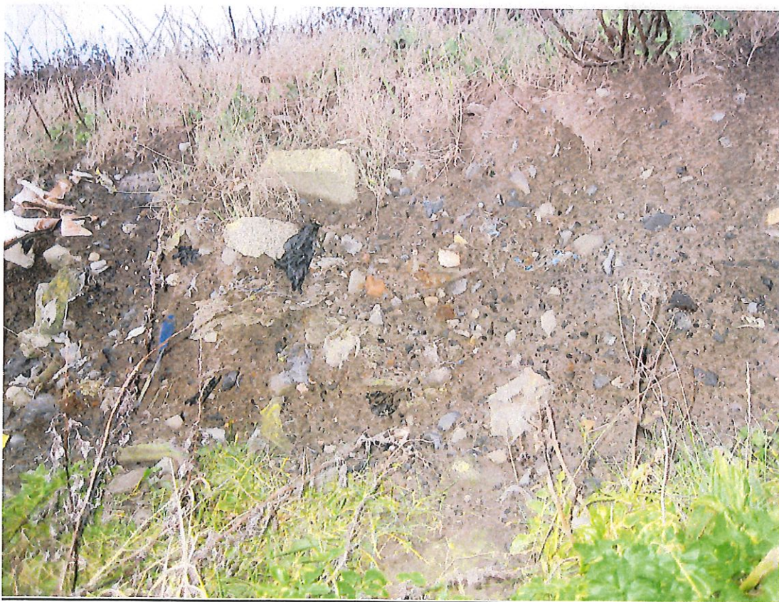
Photograph 7: Waste Exposed along Southern Face of landfill
