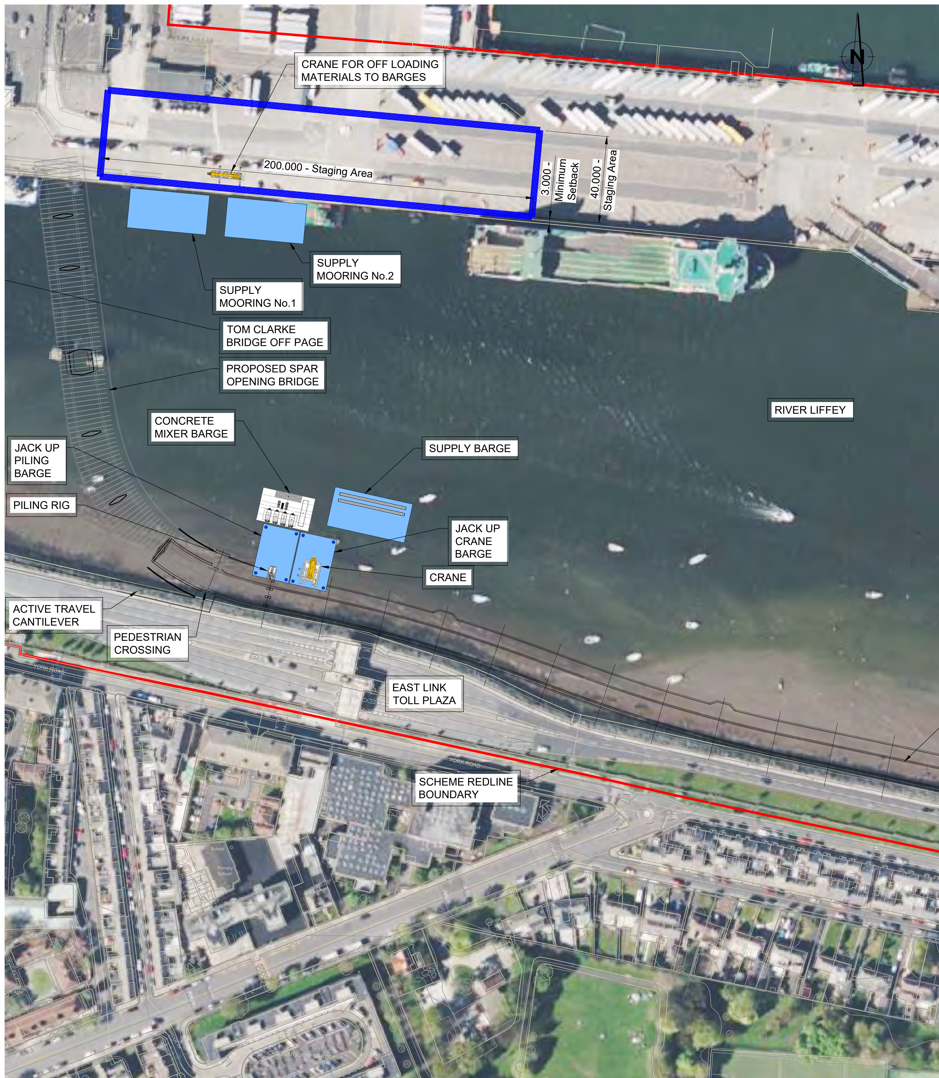
STAGE 3 - PERMANENT PILING - PLAN (Scale 1 : 1,000)
