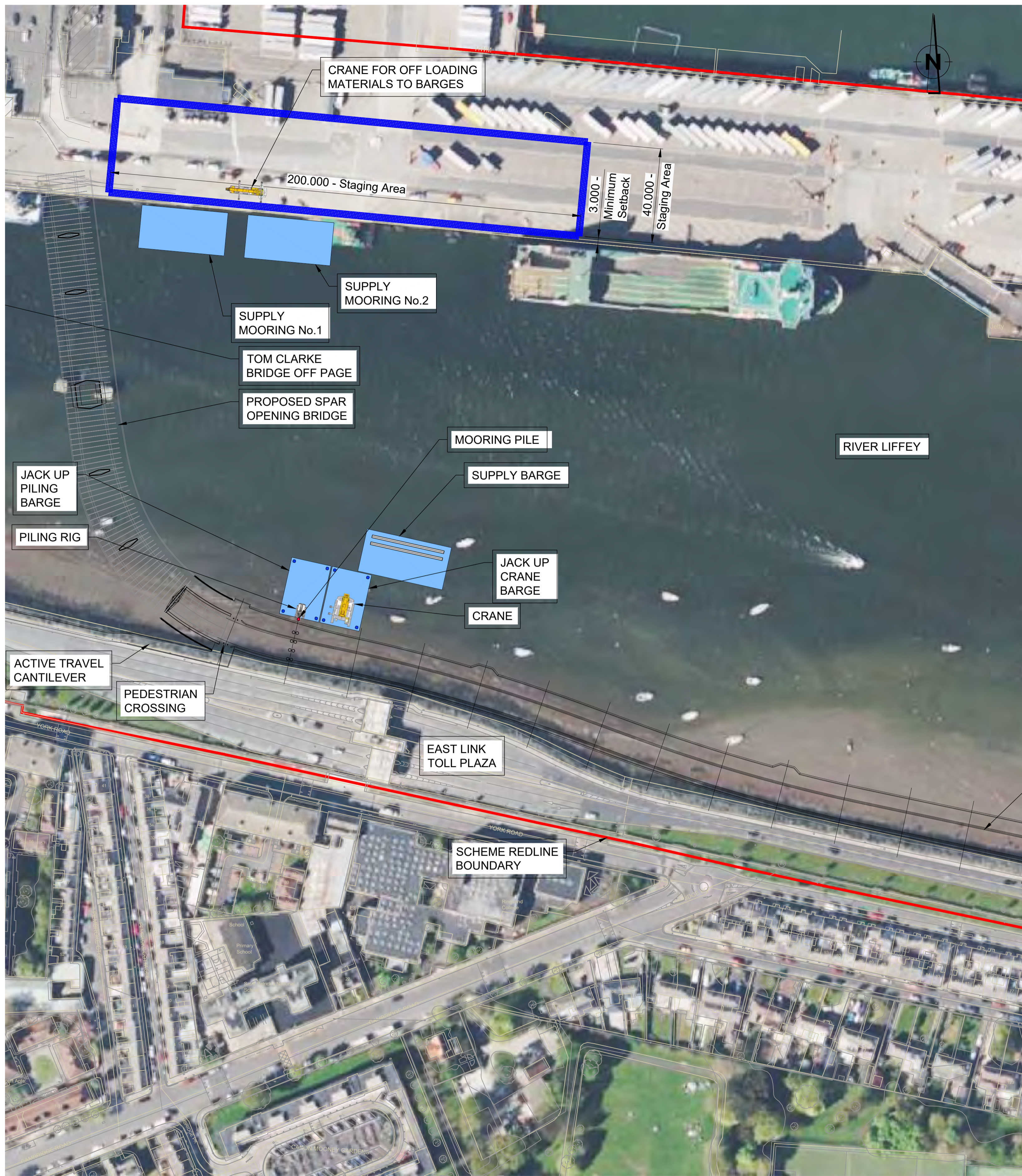
STAGE 4 - MOORING PILING - PLAN (Scale 1 : 1,000)
