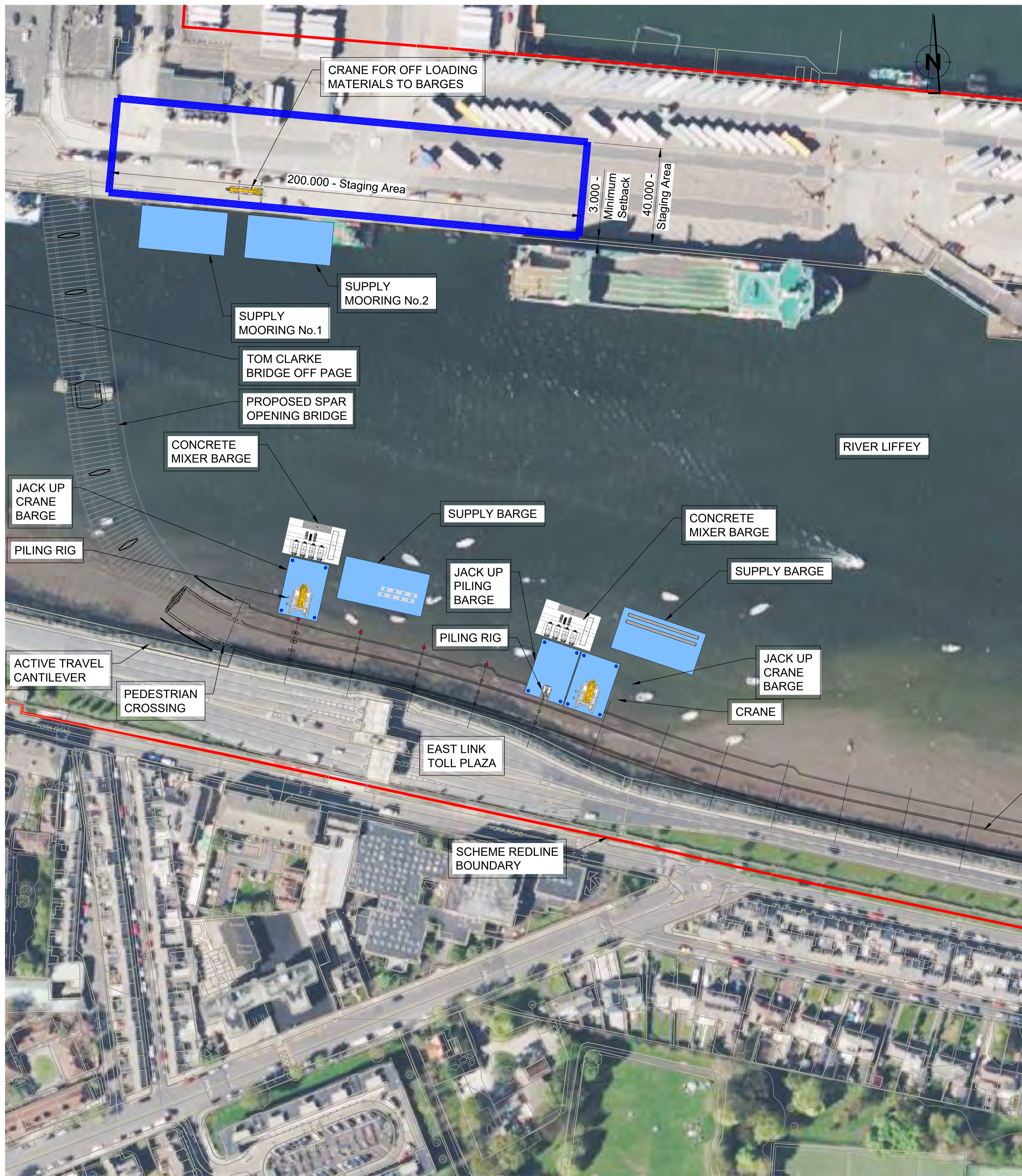
STAGE 6 - PRE-CAST CROSSHEAD INSTALLATION AND IN-SITU POUR - PLAN (Scale 1 : 1,000)
