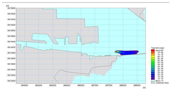
Figure 13.36: Suspended sediment concentration plume in the bottom layer during a typical mid ebb phase of a spring tidal cycle whilst dredging the berthing pocket at Area N
