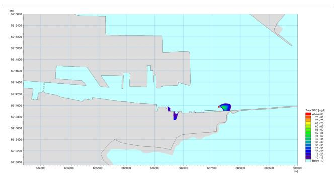
Figure 13.40: Suspended sediment concentration plume in the bottom layer during a typical high water phase of a spring tidal cycle whilst dredging construction access at Area N
