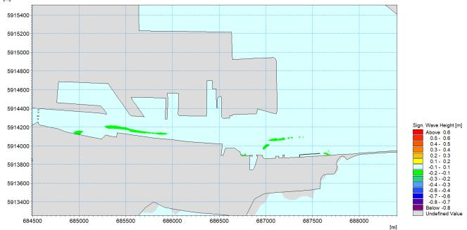
Figure 13.61: Difference in wave heights during a south easterly storm event as a result of the 3FM Project
