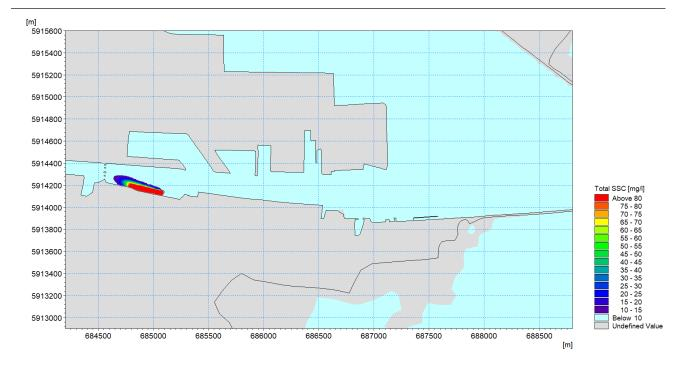
Figure 13.19: Suspended sediment concentration plume in the bottom layer during a typical mid flood phase of a spring tidal cycle whilst dredging the Maritime Village
