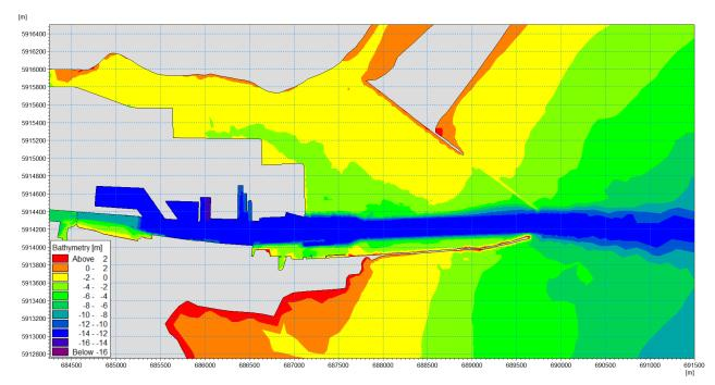
Figure 13.3: Bathymetry of the Dublin Port pre 3FM Project (post ABR & MP2 Project) model – levels illustrated to Mean Sea Level
