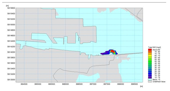
Figure 13.34: Suspended sediment concentration plume in the bottom layer during a typical mid flood phase of a spring tidal cycle whilst dredging the berthing pocket at Area N
