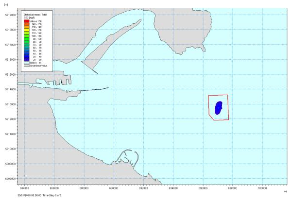
Figure 13.45: Mean Total Suspended Solids Concentration envelope using a Trailing Suction Hopper Dredger dumping circa 2,030 tonnes wet weight at 3 hourly intervals on average within each winter capital dredging season
