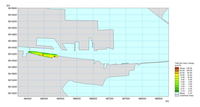
Figure 13.22: Deposition of sediment following the dredging operations at the Maritime Village
