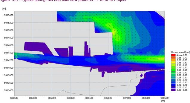
Figure 13.7: Typical spring mid ebb tidal flow patterns - Pre-3FM Project
