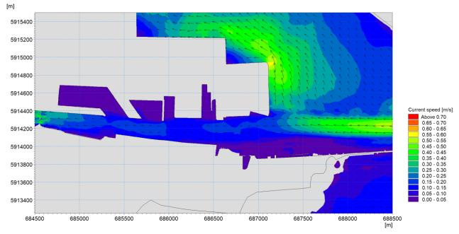
Figure 13.53: Typical spring mid flood tidal flow patterns – Post 3FM Project
