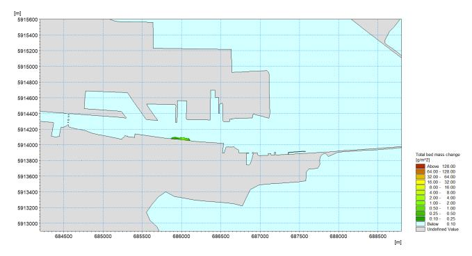
Figure 13.27: Deposition of sediment following the dredging operations at Area K
