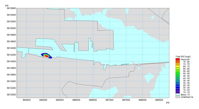
Figure 13.18: Suspended sediment concentration plume in the bottom layer during a typical low water phase of a spring tidal cycle whilst dredging the Maritime Village
