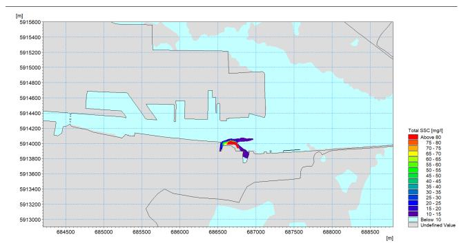
Figure 13.28: Suspended sediment concentration plume in the bottom layer during a typical low water phase of a spring tidal cycle whilst dredging the Turning Circle
