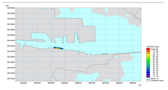
Figure 13.24: Suspended sediment concentration plume in the bottom layer during a typical mid flood phase of a spring tidal cycle whilst dredging Area K
