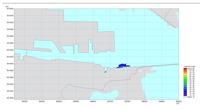
Figure 13.38: Suspended sediment concentration plume in the bottom layer during a typical low water phase of a spring tidal cycle whilst dredging construction access at Area N
