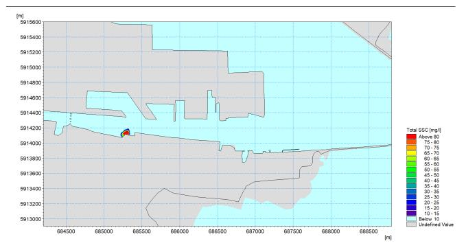
Figure 13.21: Suspended sediment concentration plume in the bottom layer during a typical mid ebb phase of a spring tidal cycle whilst dredging the Maritime Village
