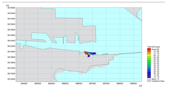
Figure 13.30: Suspended sediment concentration plume in the bottom layer during a typical high water phase of a spring tidal cycle whilst dredging Turning Circle
