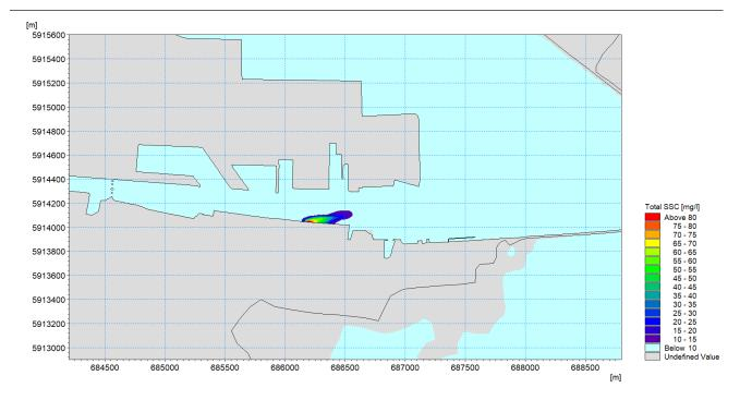
Figure 13.26: Suspended sediment concentration plume in the bottom layer during a typical mid ebb phase of a spring tidal cycle whilst dredging Area K
