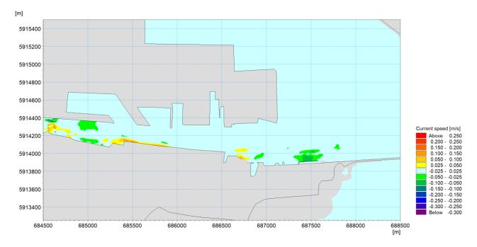
Figure 13.55: Difference in typical spring mid flood tidal flow patterns as a result of the 3FM Project
