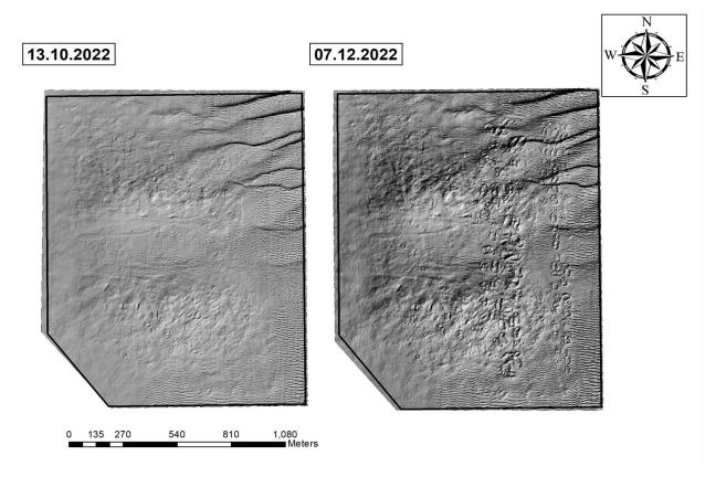
Figure 13.49: Sand wave and other morphological features identified from a terrain analyses of both survey datasets
