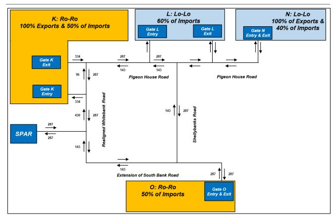
Figure 14.65 Schematic of HGV Traffic Flows for Ro-Ro Terminal -8 Hour (23:00-07:00) - Unit Vehicles
