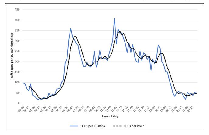
Figure 14.42 Existing Circle K Roundabout Daily Profile of the total turning movements
