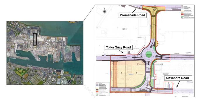
Figure 14.11 T10 Link Road Extension Proposed Location and Layout (DCC Planning Ref. No.: 4894/22)
