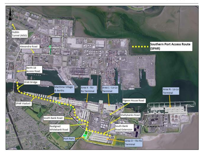
Figure 14.13 3FM Project Preliminary General Arrangement Layout (May 2024)
