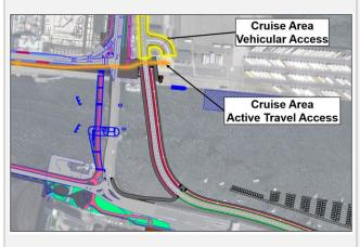
The proposed Berth 18 Access Road will give vehicular access to the Cruise berth, and active travel users will access the berth via a proposed demand controlled (i.e. signalised) crossing of the SPAR and through the North Wall Square public realm area.
