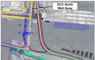
The Point Junction Improvement Scheme is a DCC proposal to replace the existing Point roundabout with a signalised junction and provide improved pedestrian and cycling facilities along East Wall Road.
