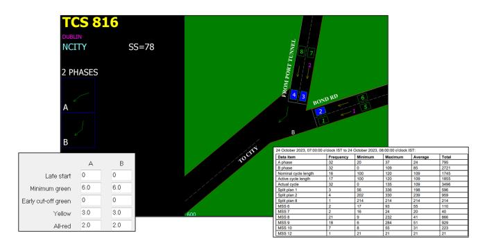
Figure 14.38 Example of DCC Data from the Traffic Signal Controller at Junction 8
