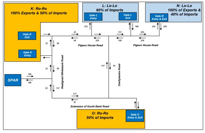
Figure 14.51 Schematic of HGV Traffic Flows for Lo-Lo Terminal – Worst Case Peak Hour – Unit PCUS
