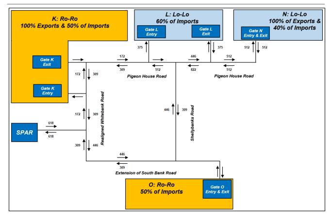
Figure 14.53 Schematic of HGV Traffic Flows for Lo-Lo Terminal –16 Hour (07:00-23:00) – Unit Vehicles
