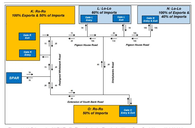
Figure 14.50 Schematic of HGV Traffic Flows for Lo-Lo Terminal – Worst Case Peak Hour – Unit Vehicles
