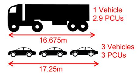
Figure 14.43 Illustration of OGV2 at 2.9PCU Conversion Rate
