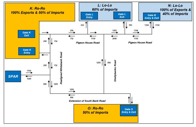
Figure 14.54 Schematic of HGV Traffic Flows for Lo-Lo Terminal – 16 Hour (07:00-23:00) – Unit PCUS
