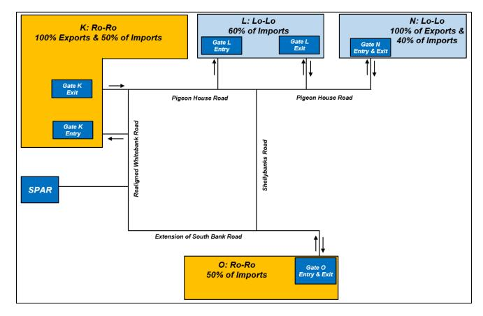
Figure 14.20 Schematic of Land Use, Location and Access Arrangements for HGVs to Areas K, L, N & O
