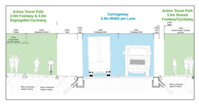
Figure 14.97 Proposed SPAR Cross Section
