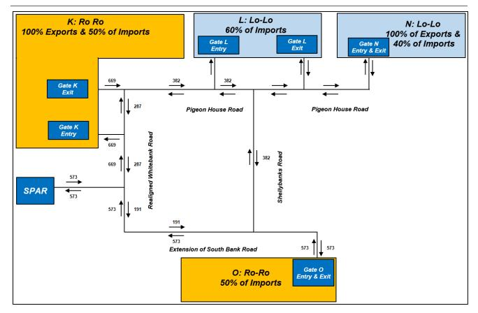
Figure 14.62 Schematic of HGV Traffic Flows for Ro-Ro Terminal –16 Hour (07:00-23:00) – Unit Vehicles
