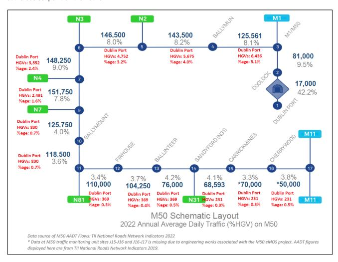
Figure 14.6 Schematic showing overall vehicle numbers across the M50 in 2022. Dublin Port related HGV figures and percentages of overall vehicles are in red
