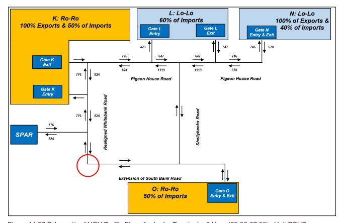
Figure 14.57 Schematic of HGV Traffic Flows for Lo-Lo Terminal – 8 Hour (23:00-07:00) – Unit PCUS
