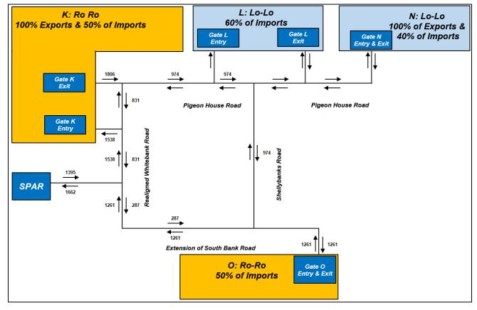
Figure 14.63 Schematic of HGV Traffic Flows for Ro-Ro Terminal – 16 Hour (07:00-23:00) – Unit PCUS
