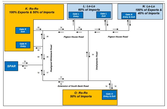
Figure 14.59 Schematic of HGV Traffic Flows for Ro-Ro Terminal – Worst Case Peak Hour – Unit Vehicles
