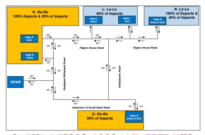
Figure 14.66 Schematic of HGV Traffic Flows for Ro-Ro Terminal – 8 Hour (23:00-07:00) – Unit PCUS
