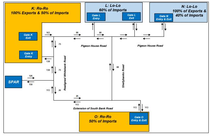
Figure 14.60 Schematic of HGV Traffic Flows for Ro-Ro Terminal – Worst Case Peak Hour – Unit PCUS
