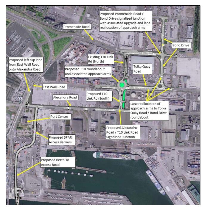
Figure 14.14 North Port Road Upgrade Works
