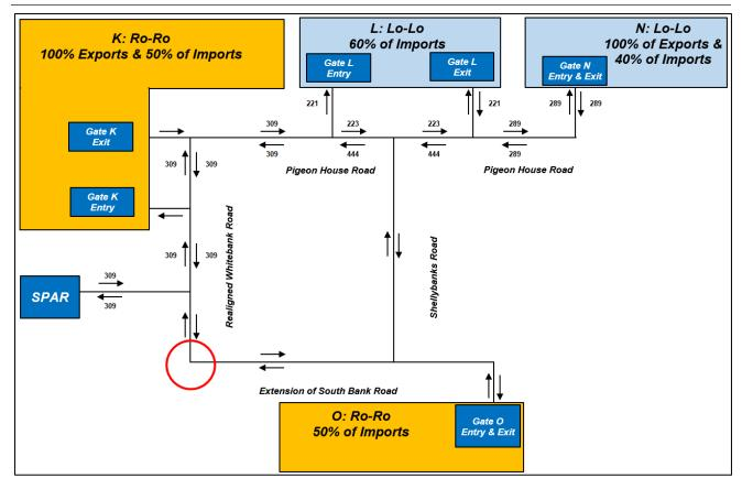
Figure 14.56 Schematic of HGV Traffic Flows for Lo-Lo Terminal –8 Hour (23:00-07:00) – Unit Vehicles
