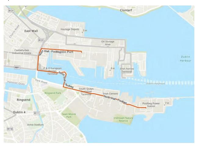
Figure 15.2 Route of the existing 220kV cable between Poolbeg and North Wall
