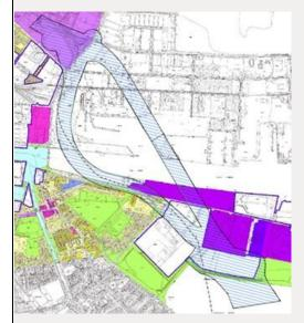
**2009:** NRA progressed a Corridor Protection Study for Sector A of the DEB, which protected these two corridors (as indicated in the image extracted from the report). The corridor to the west was for a cut & cover tunnel, and the corridor to the east for a high-level skew bridge.
