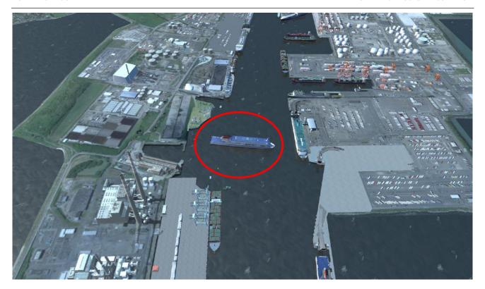
Figure 5.21 Example visual scene from HR Wallingford's Ship Simulator, illustrating the Turning Circle in use. Turning Circle shown indicatively in red. View looking west.
