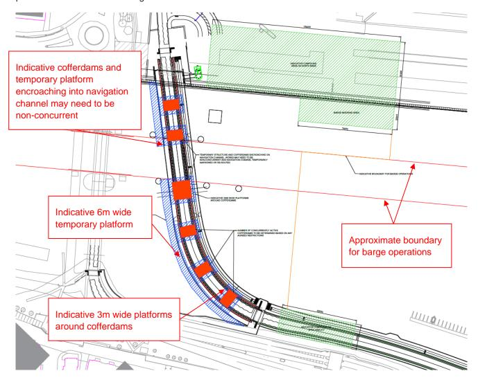
Figure 5.12 Illustrative example of temporary works for River Liffey crossing, extract from Drawing COWI-SBR-SP-DR-S-100-00090, Rev 0, Temporary Works Arrangement
