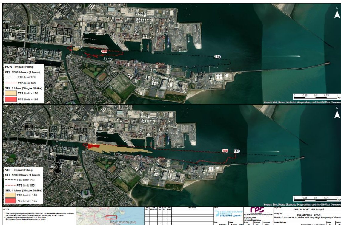
Figure 7.86 Model outputs for impact piling for 1200 blows in one hour (one blow every 3 seconds) including PTS (red) and TTS (brown) exposure for seals (PCW) and harbour porpoise (VHF) (from Chapter 12: Noise and Vibration) at SPAR Bridge.
