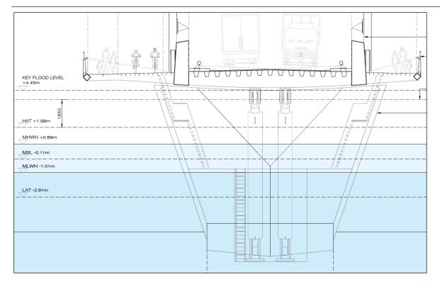
Figure 9-36 Extract from SPAR Bridge Typical Cross Section
