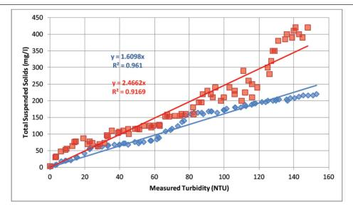
Figure 9-20 TSS versus Turbidity for suspensions of river bed silt sediment (red) and approach channel fine sand sediment (blue). Equations and r<sup>2</sup> values are shown in corresponding colours for each series.
