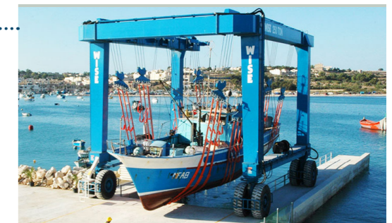
▲ Mobile Boat Hoist on Finger Piers
