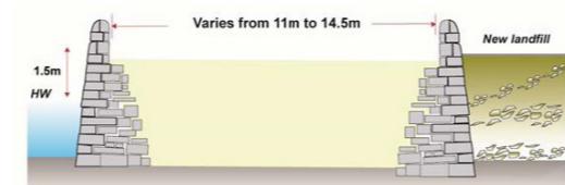
▲ GSW Cross section between Pigeon House precinct and Ringsend (Drawn at exposed section near disused sewerage outfall) Source: Southgate for DPC
