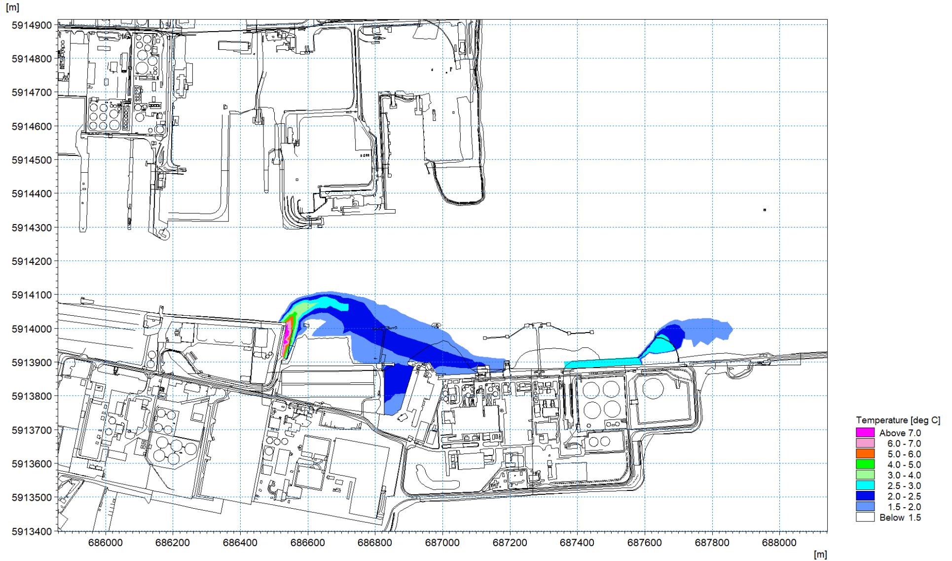
Figure 1.82: Thermal plume 20 th April 2018 – excess temperature at mid-flood circa 0.3m depth layer 6
