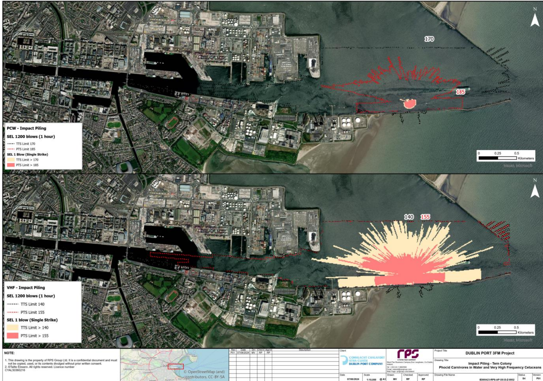
Figure 12.2.35. Impact piling, Tern Colony, VHF and PCW hearing group.
