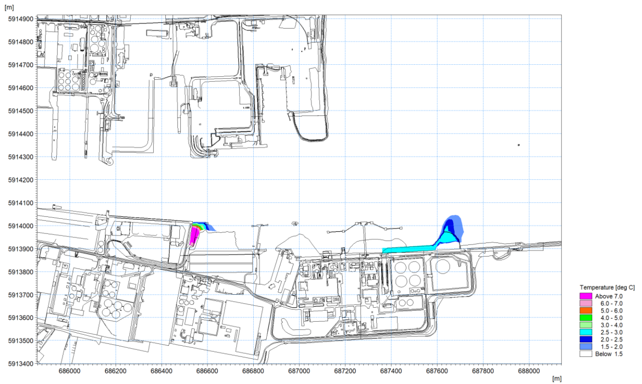
Figure 1.19: Thermal plume 20 th April 2018 – excess temperature at mid-flood circa 0.3m depth.
