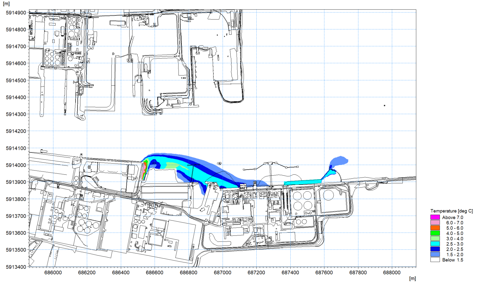
Figure 1.104: Thermal plume 24 th April 2018 – excess temperature at low water circa 1m depth layer 5
