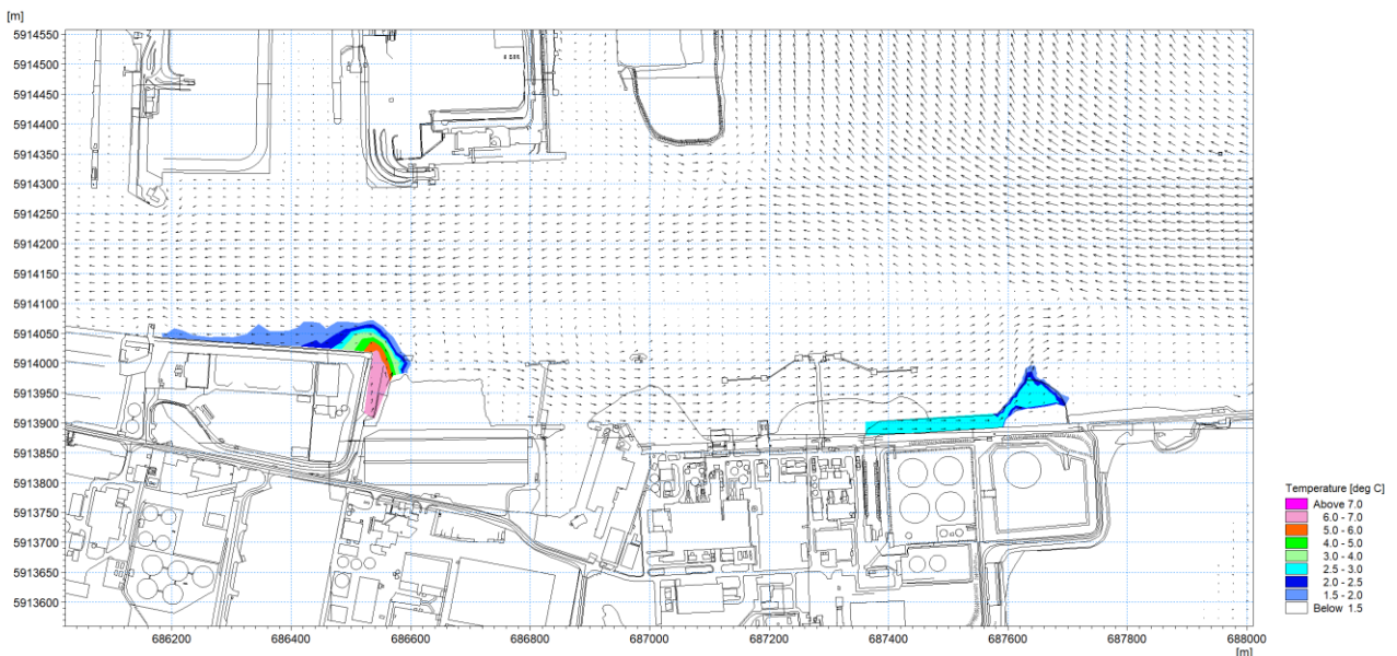
Figure 1.40: Thermal plume 20 th April 2018 – excess temperature at low water circa 2m depth.
