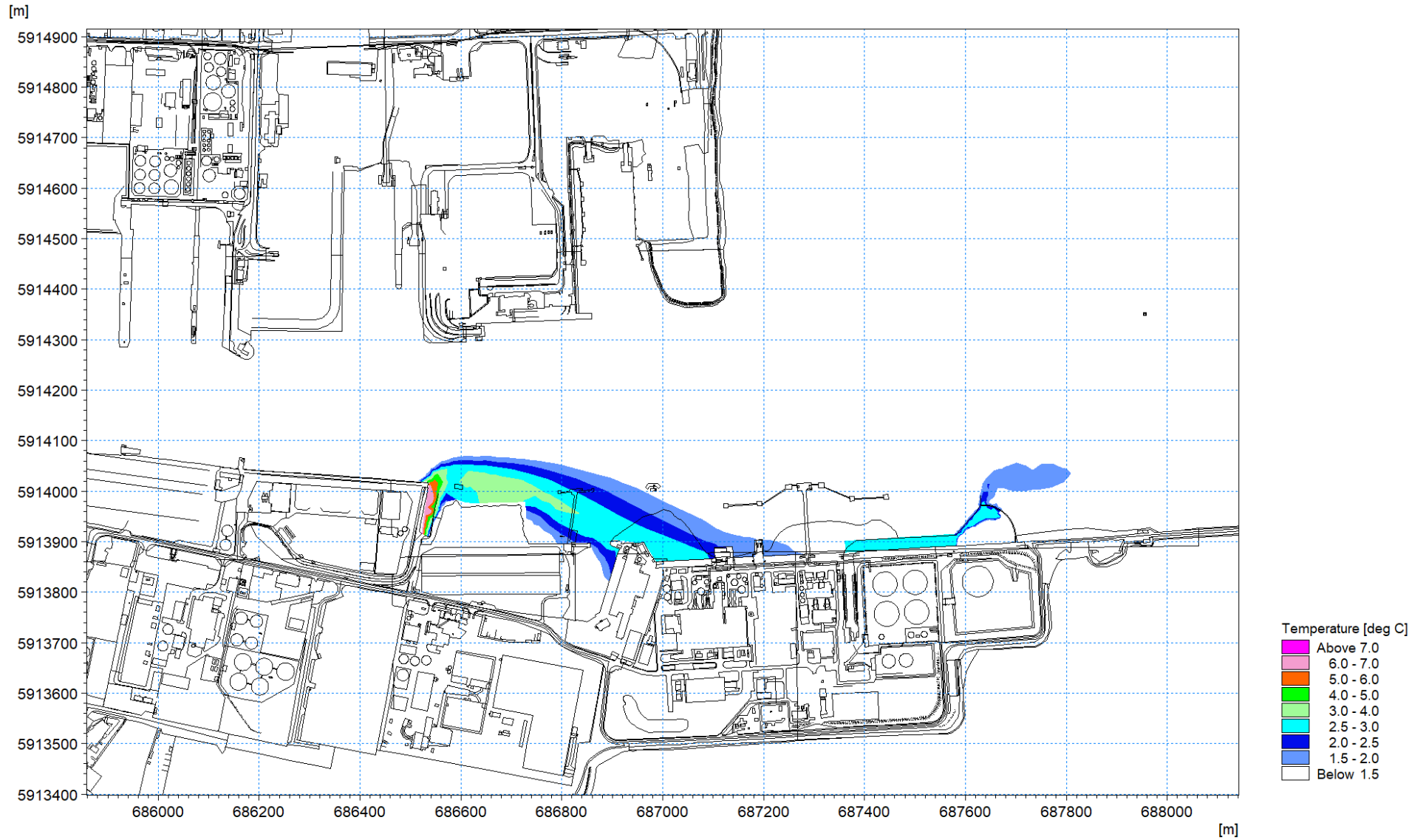
Figure 1.103: Thermal plume 24 th April 2018 – excess temperature at low water circa 0.3m depth layer 6
