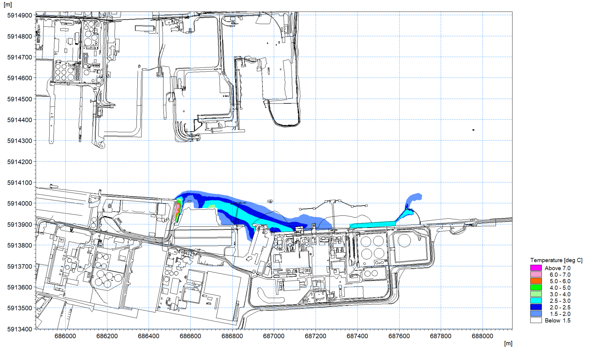
Figure 1.105: Thermal plume 24 th April 2018 – excess temperature at low water circa 2m depth layer 4
