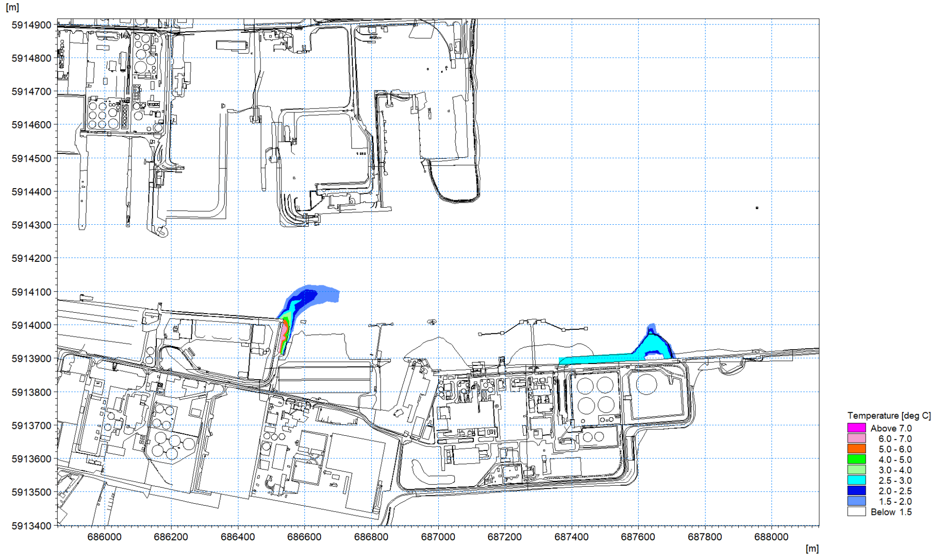
Figure 1.98: Thermal plume 24 th April 2018 – excess temperature at high water circa 1m depth layer 5
