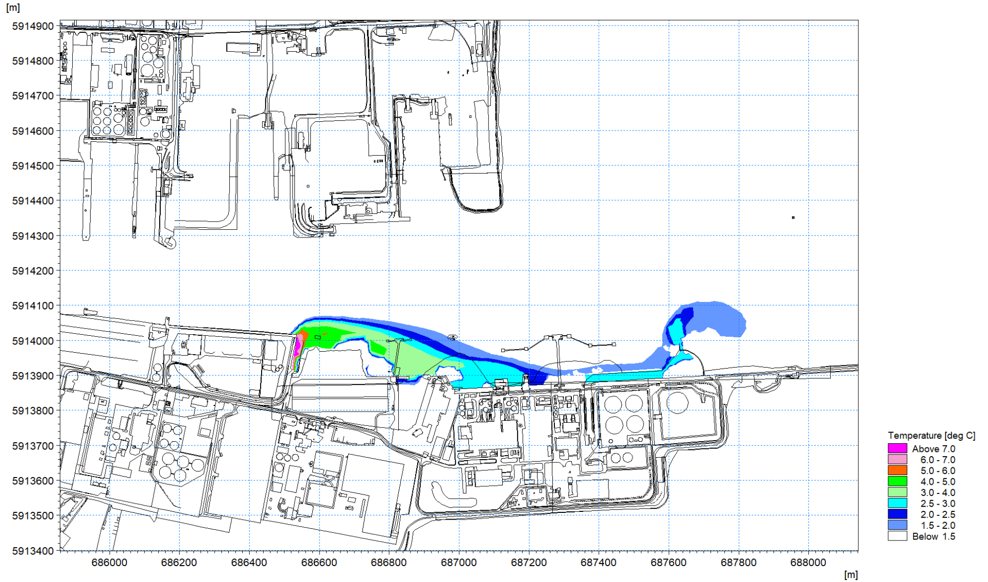
Figure 1.91: Thermal plume 20 th April 2018 – excess temperature at low water circa 0.3m depth layer 6
