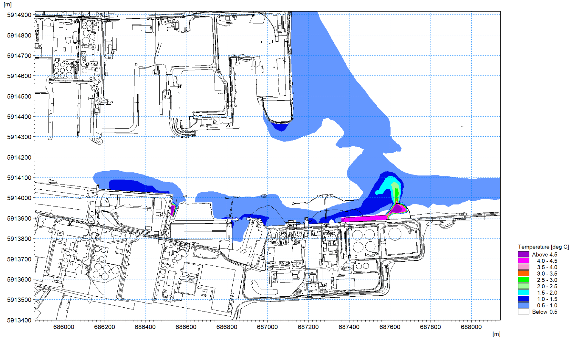
Figure 1.115: Thermal plume 9 th April 2019 – excess temperature at low water circa 1.8m depth
