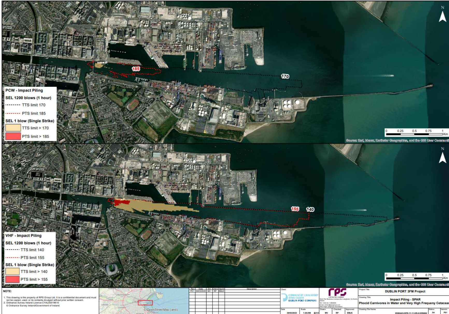
Figure 12.2.13. Impact piling, SPAR Bridge, VHF and PCW hearing group.
