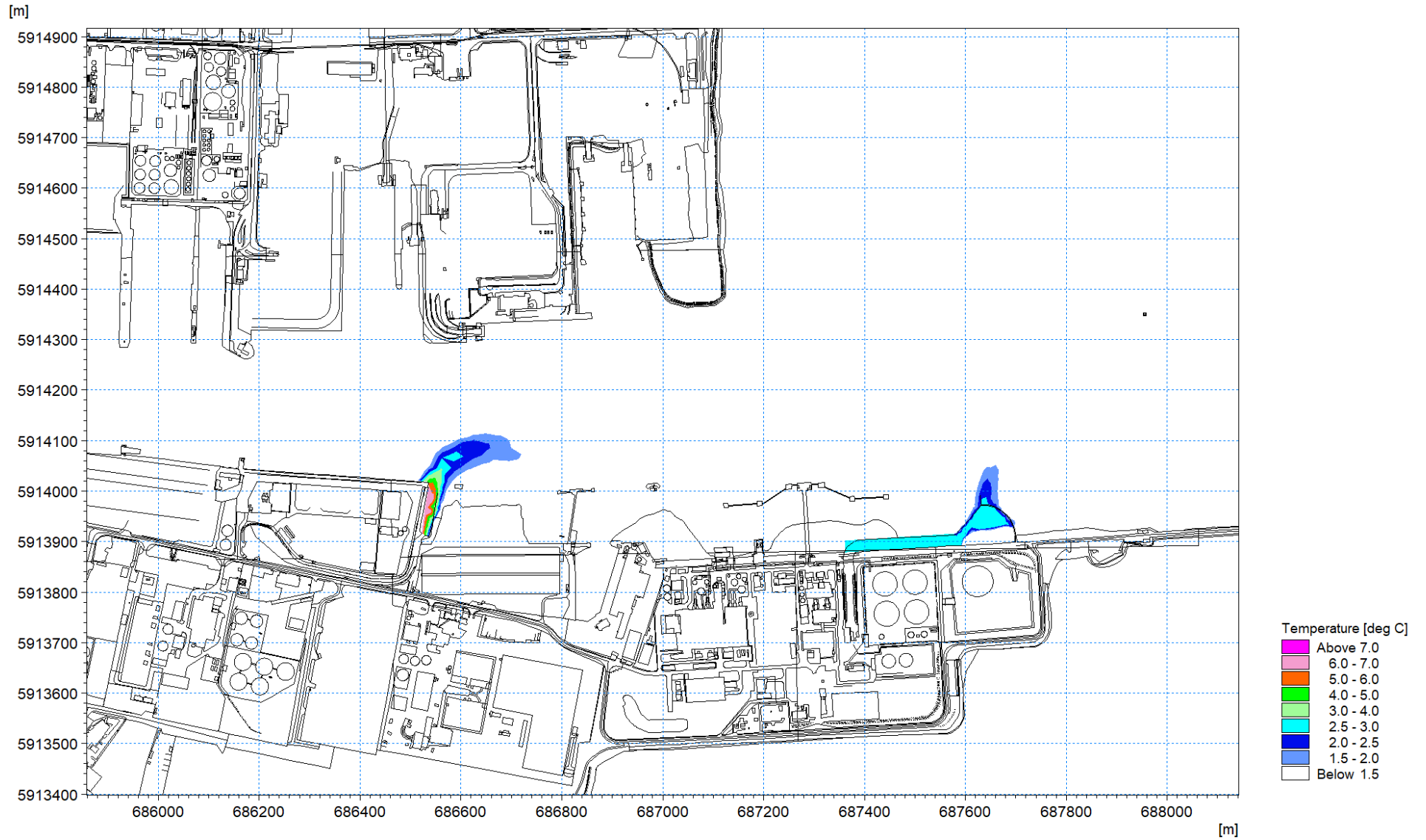
Figure 1.101: Thermal plume 24 th April 2018 – excess temperature at mid-ebb circa 1m depth layer 5
