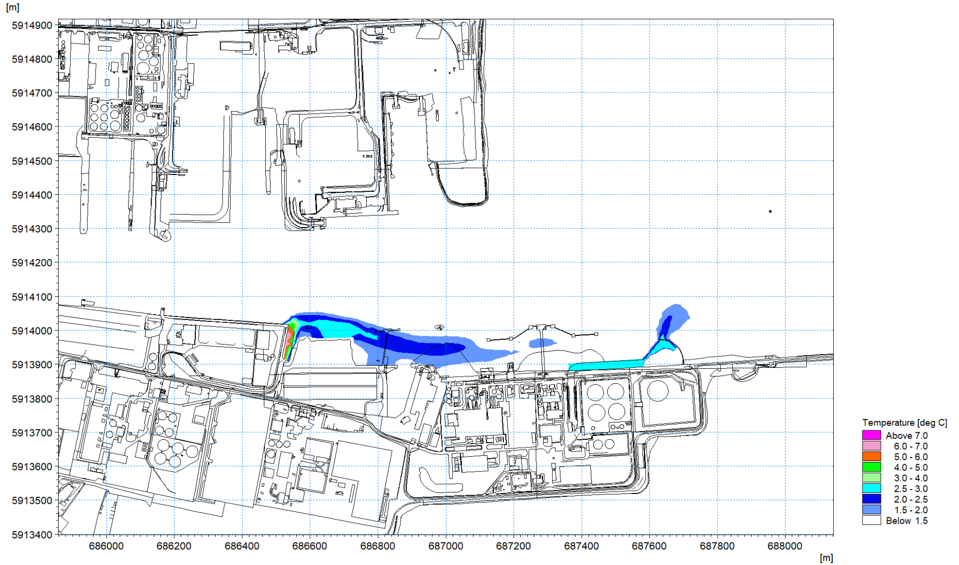
Figure 1.77: Thermal plume 12 th August 2016 – excess temperature at low water circa 1m depth layer 5
