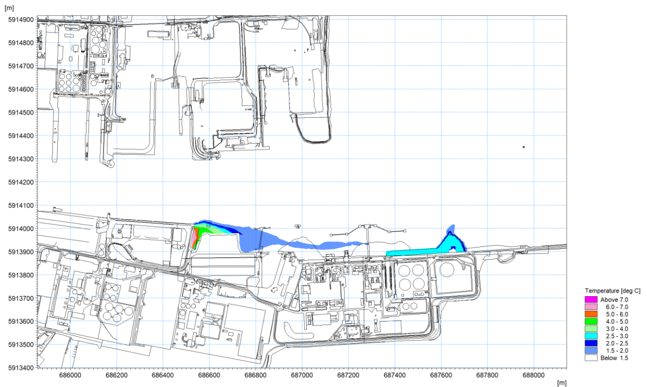
Figure 1.24: Thermal plume 20 th April 2018 – excess temperature at high water circa 1m depth.
