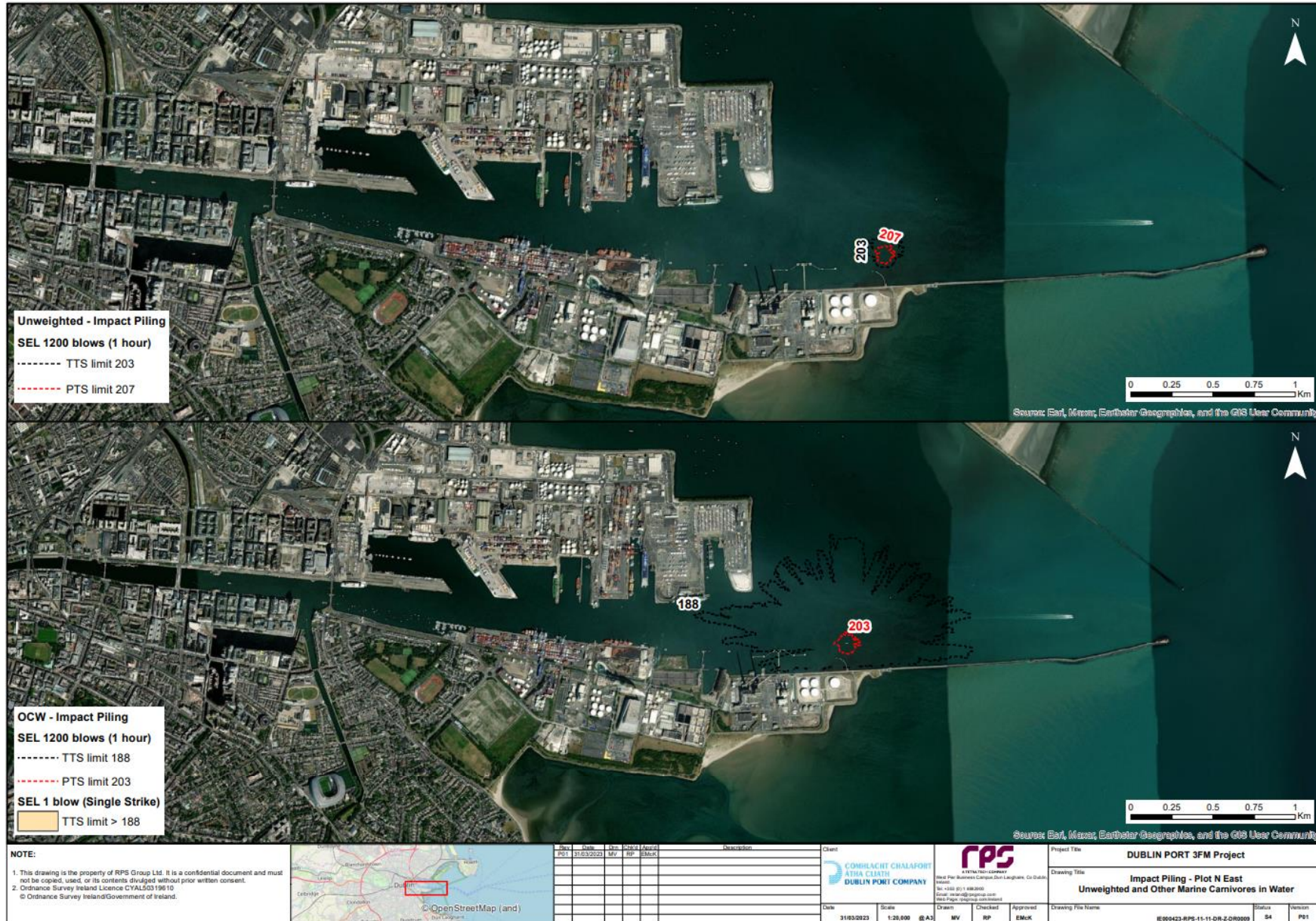
Figure 12.2.24. Impact piling, Area N east, Single piling rig, Fish (unweighted) and OCW hearing group.
