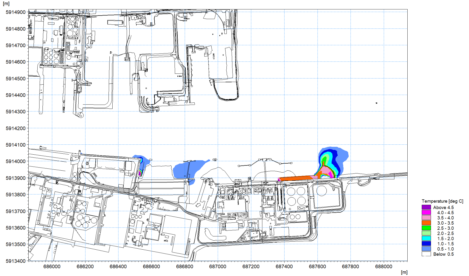
Figure 1.118: Thermal plume 9 th April 2019 – excess temperature at mid-flood circa 1.8m depth layer 4
