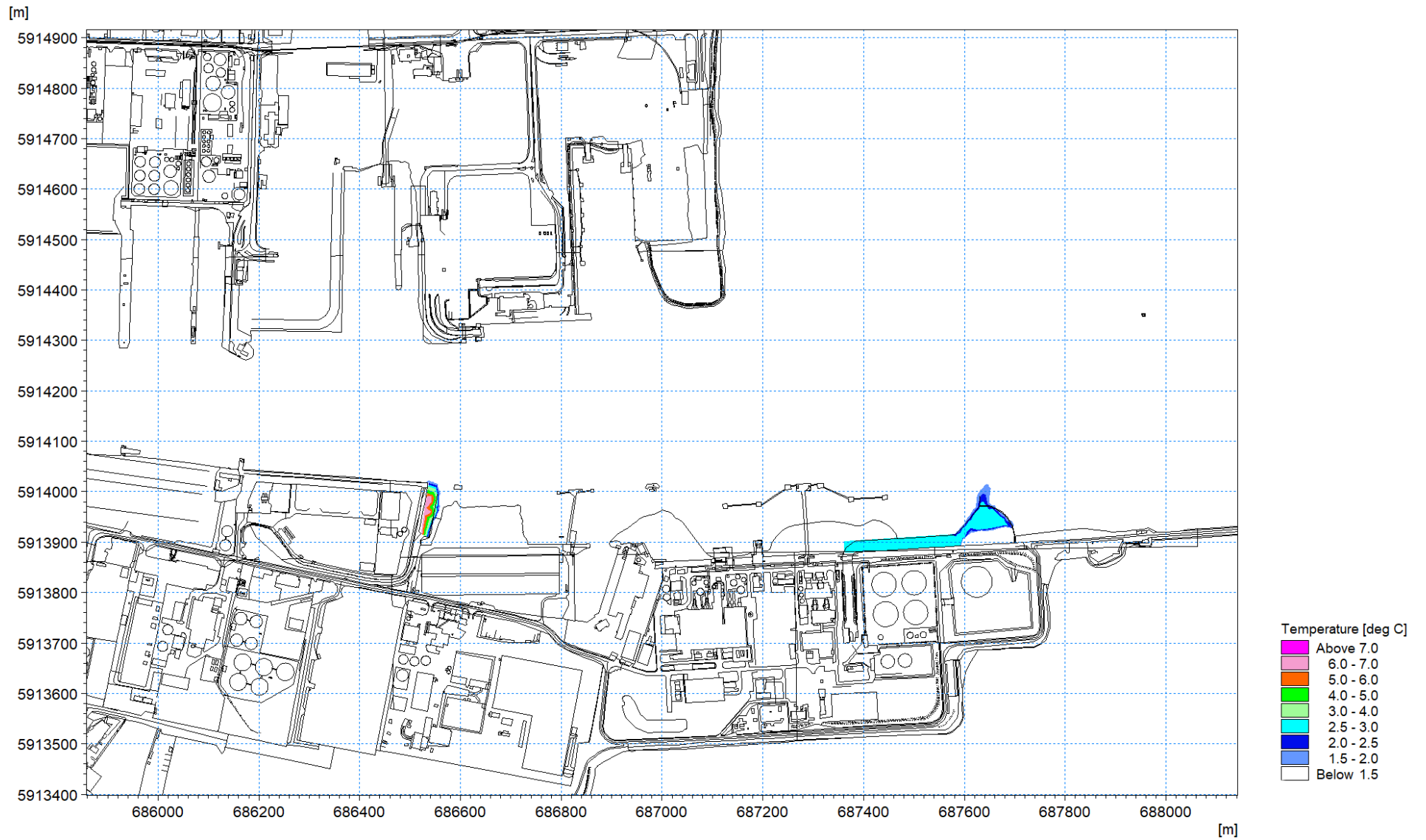
Figure 1.102: Thermal plume 24 th April 2018 – excess temperature at mid-ebb circa 2m depth layer 4
