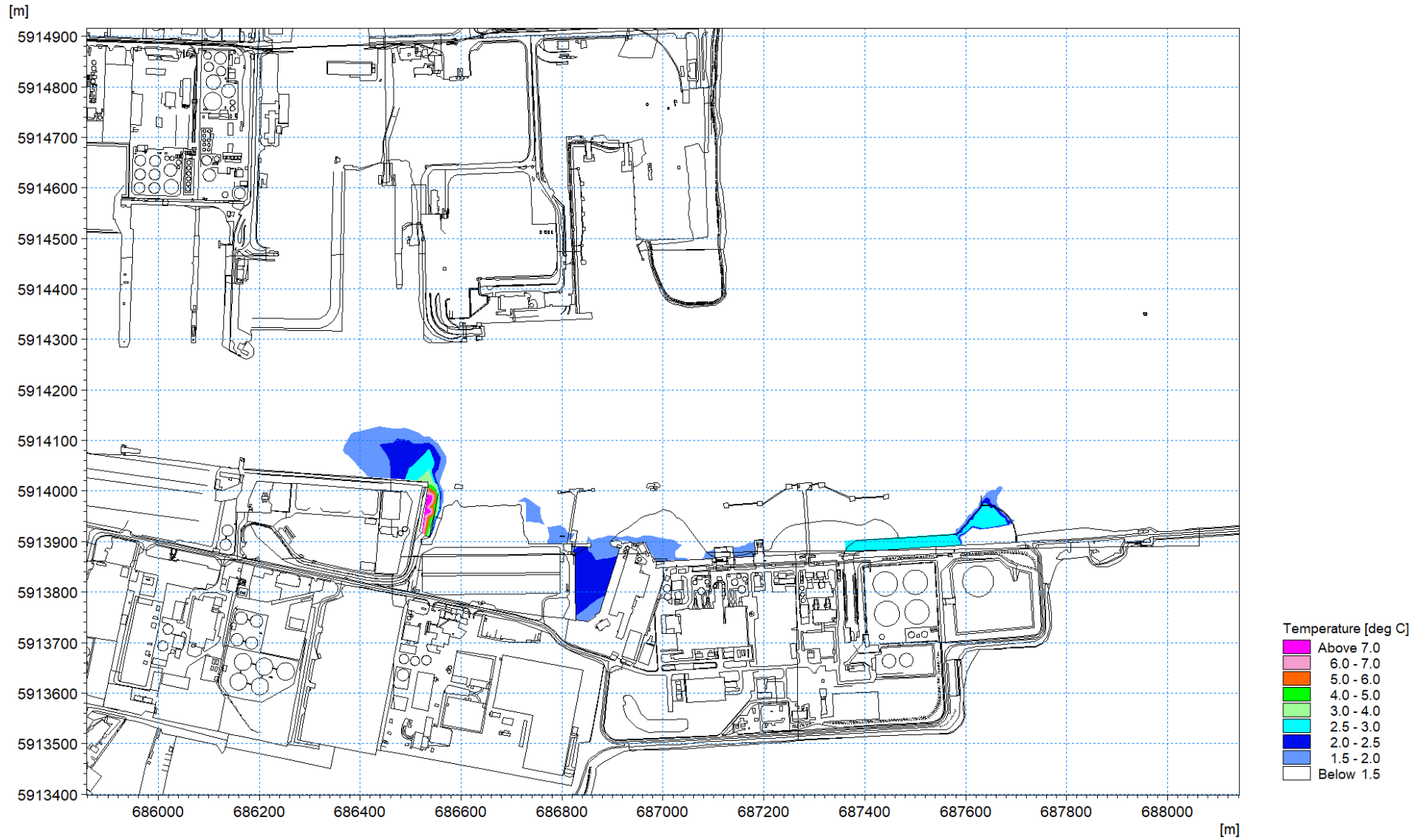
Figure 1.84: Thermal plume 20 th April 2018 – excess temperature at mid-flood circa 2m depth layer 4
