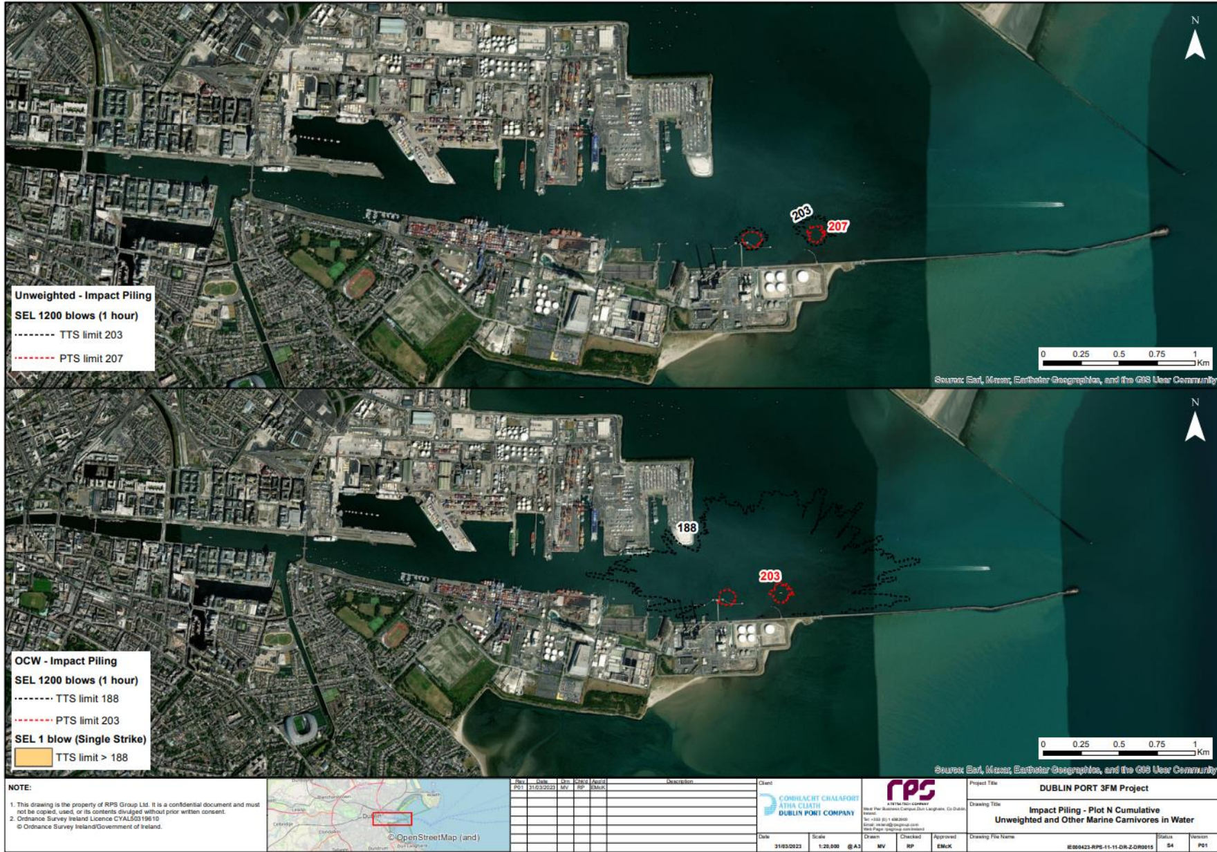
Figure 12.2.26. Impact piling, Area N west + east, two piling rigs, Fish (unweighted) and OCW hearing group.
