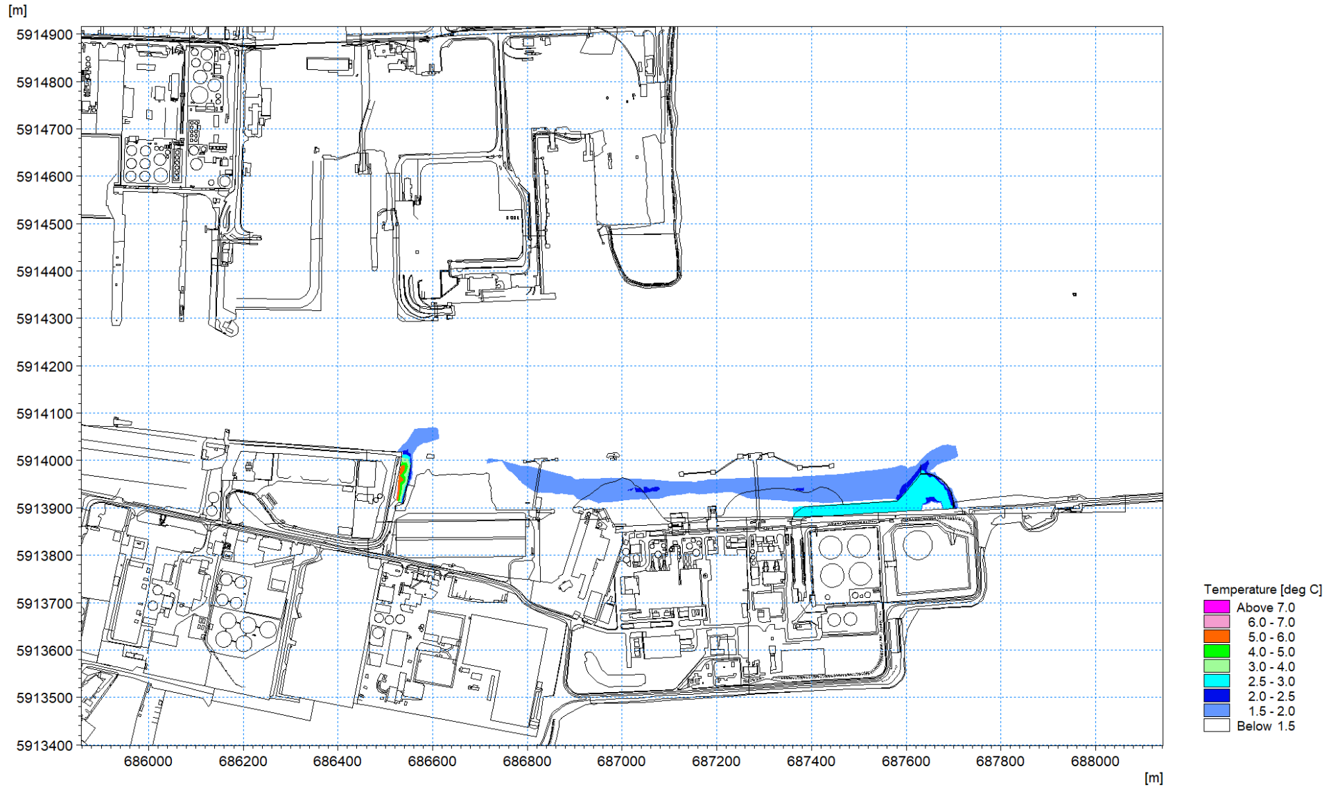
Figure 1.87: Thermal plume 20 th April 2018 – excess temperature at high water circa 2m depth layer 4
