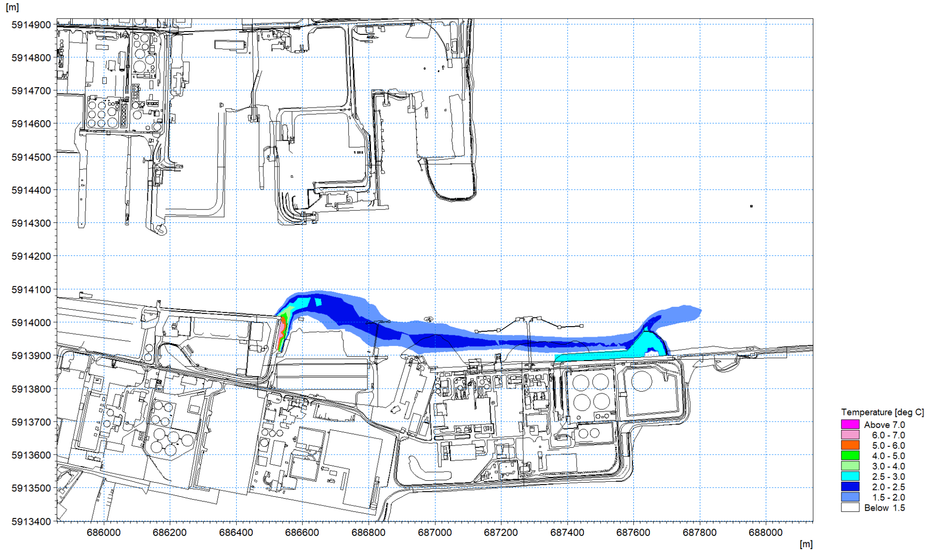
Figure 1.86: Thermal plume 20 th April 2018 – excess temperature at high water circa 1m depth layer 5
