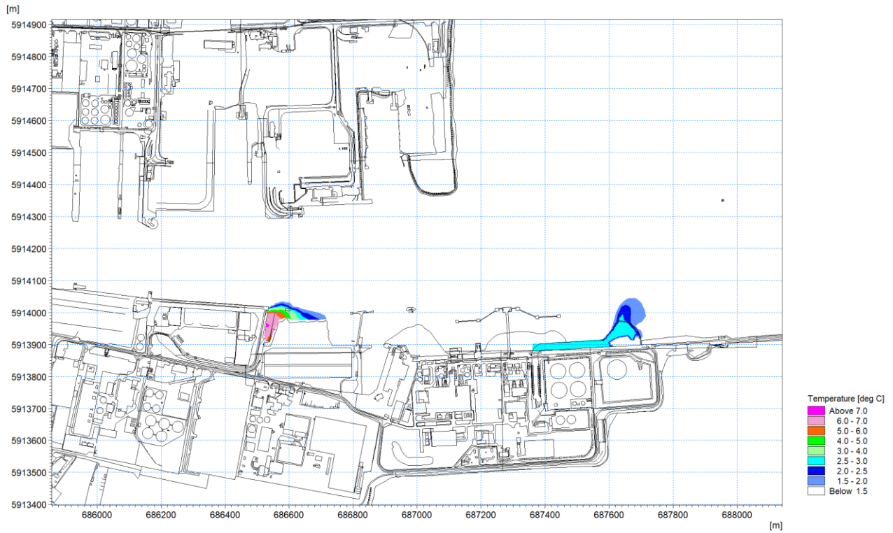
Figure 1.27: Thermal plume 20 th April 2018 – excess temperature at mid-ebb circa 0.3m depth.
