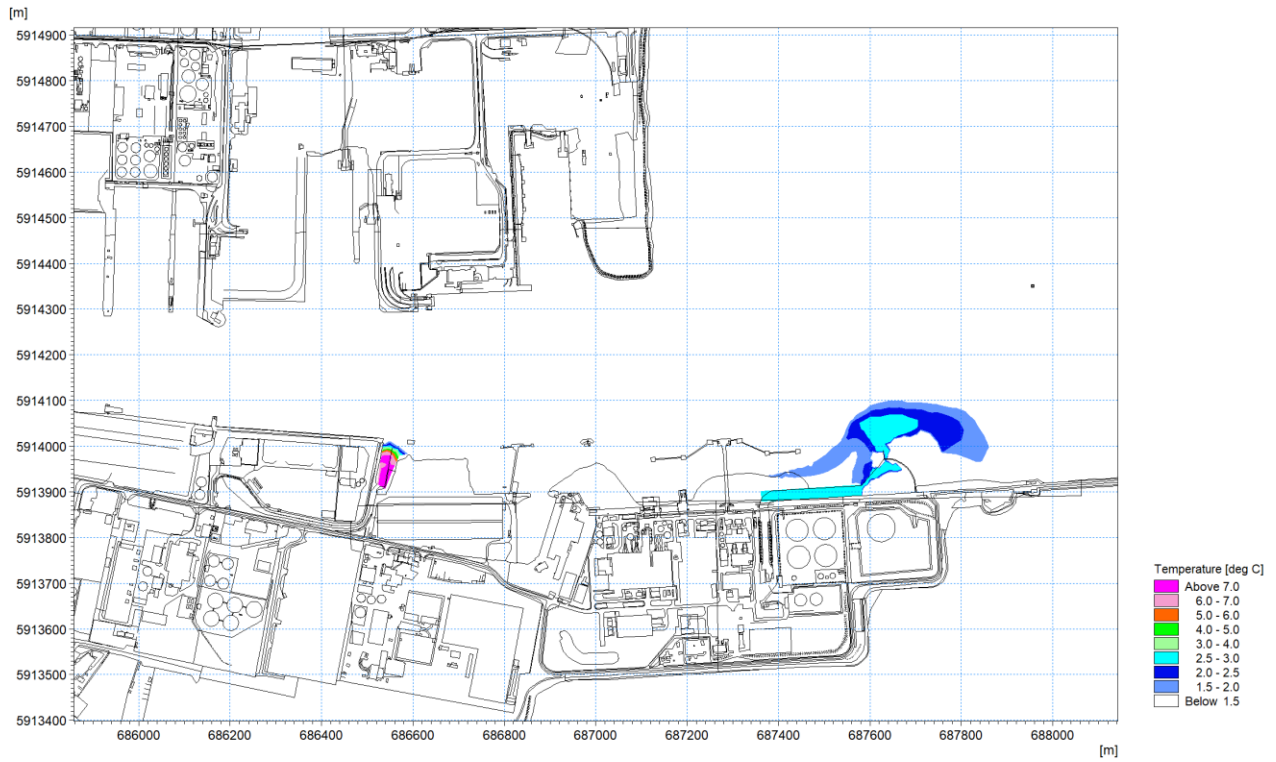
Figure 1.31: Thermal plume 20 th April 2018 – excess temperature at low water circa 0.3m depth.
