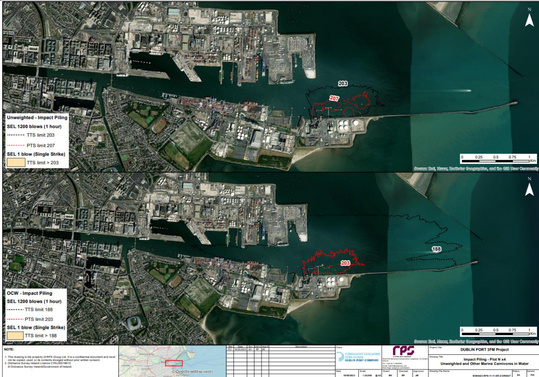
Figure 12.2.28. Impact piling, Area N, five piling rigs, Fish (unweighted) and OCW hearing group.
