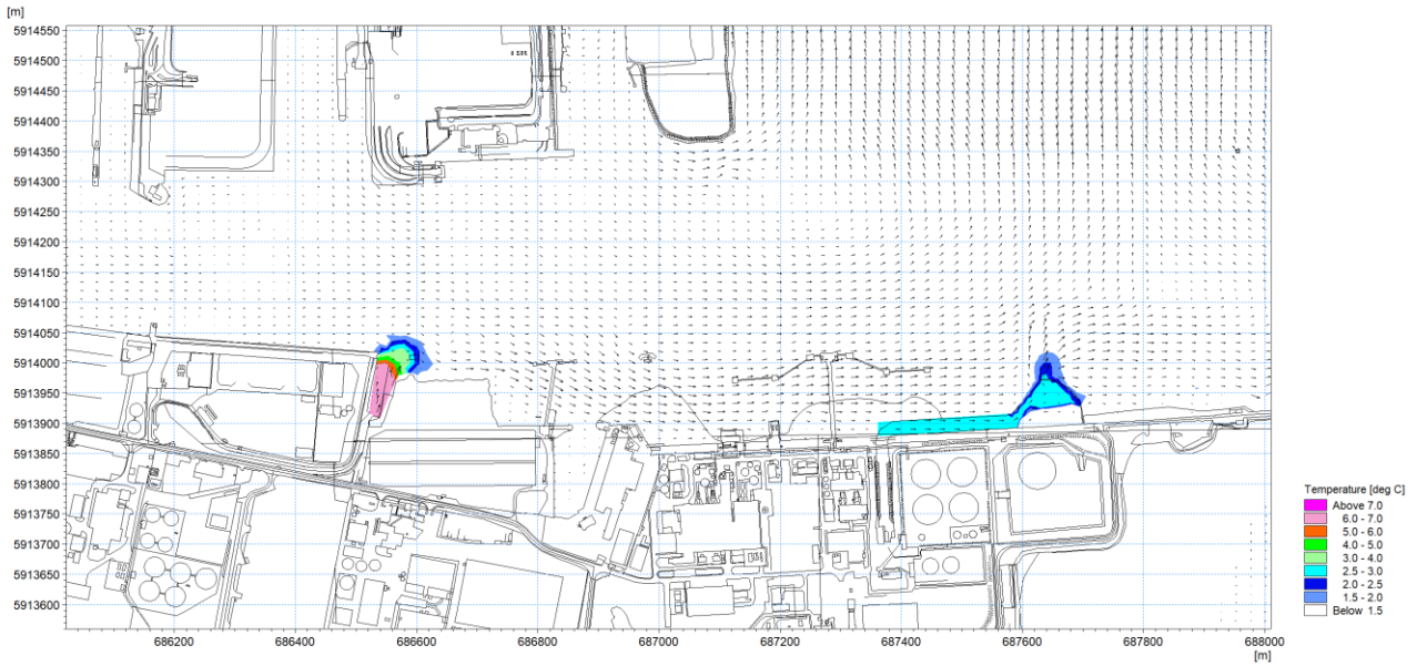
Figure 1.39: Thermal plume 24 th April 2018 – excess temperature at mid-flood circa 1m depth.
