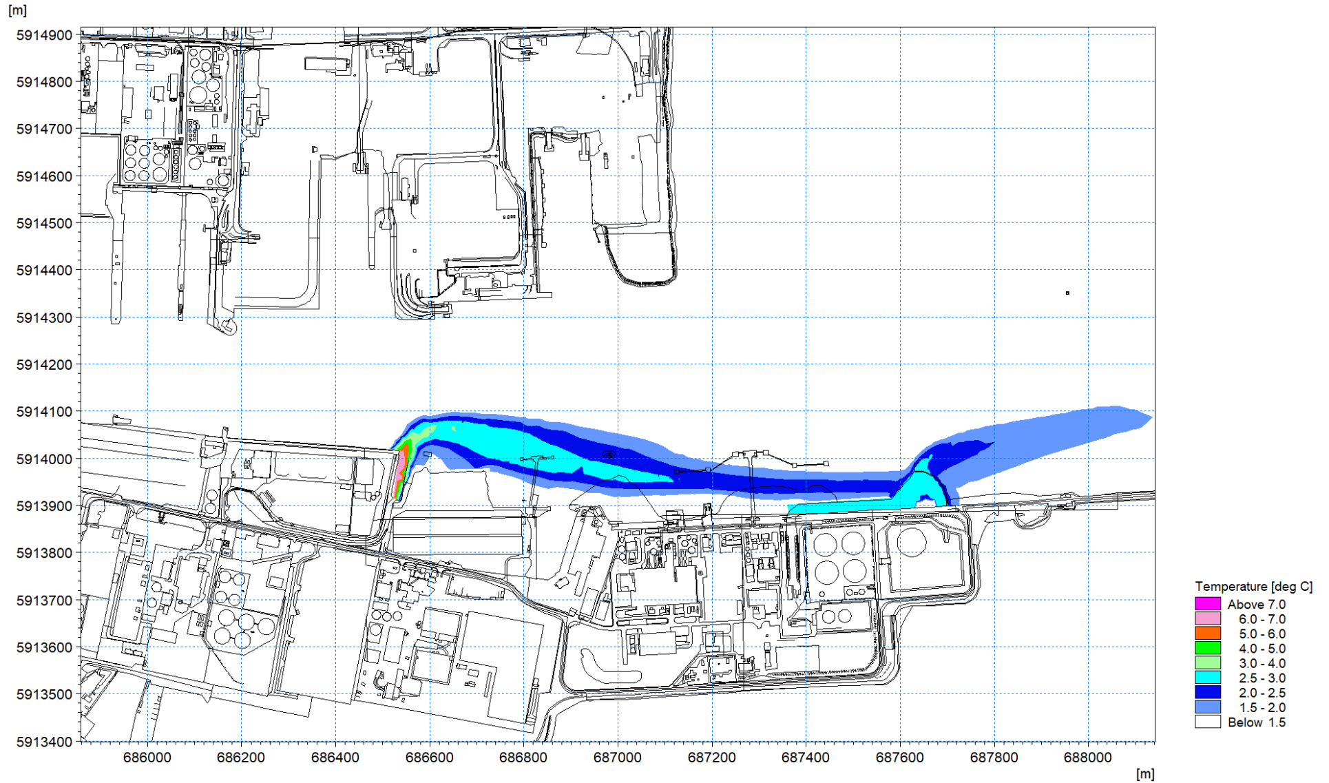
Figure 1.85: Thermal plume 20 th April 2018 – excess temperature at high water circa 0.3m depth layer 6
