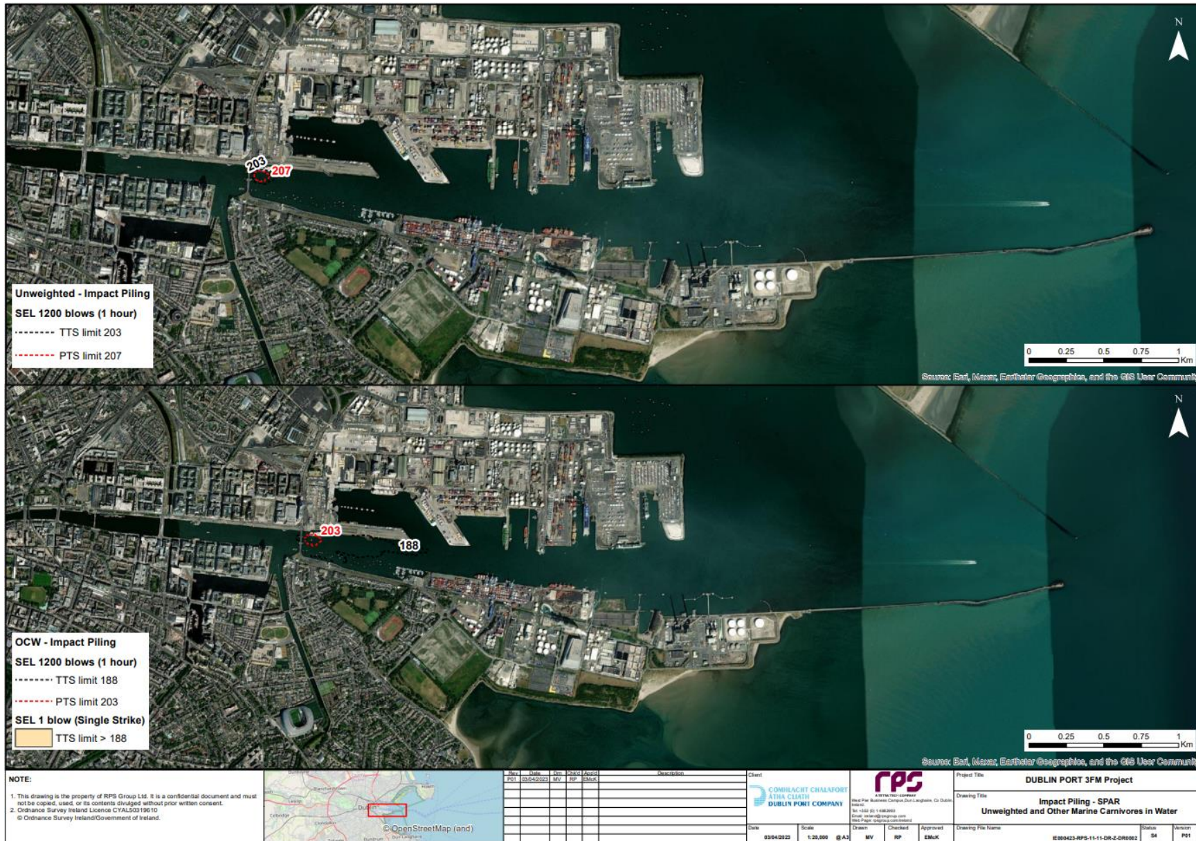
Figure 12.2.12. Impact piling, SPAR Bridge, Fish (unweighted) and OCW hearing group.
