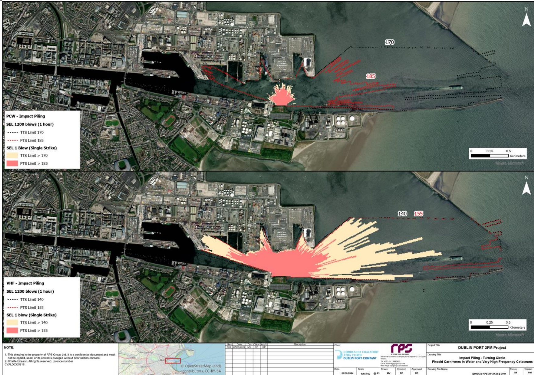
Figure 12.2.33. Impact piling, Turning circle, VHF and PCW hearing group.
