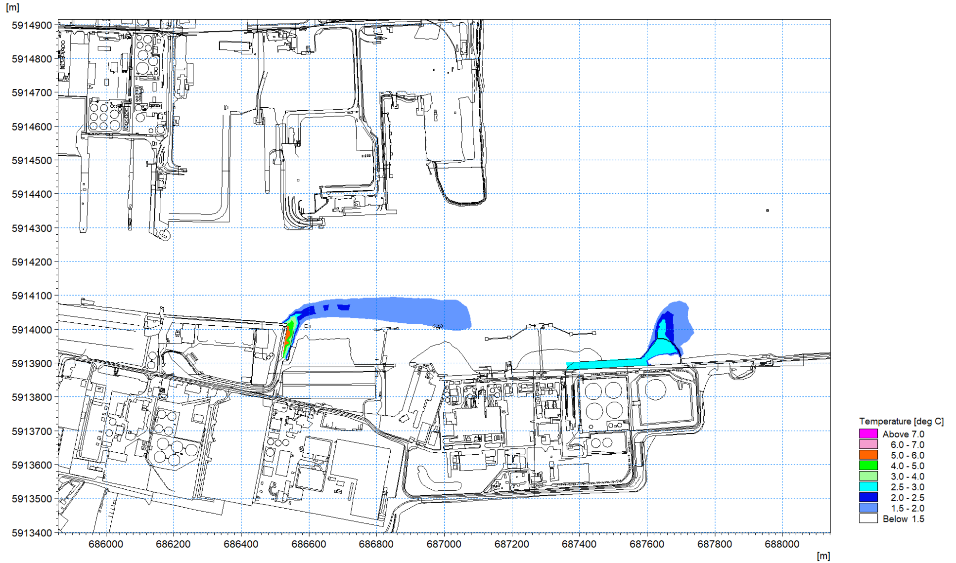
Figure 1.70: Thermal plume 12 th August 2016 – excess temperature at high water circa 0.3m depth layer 6
