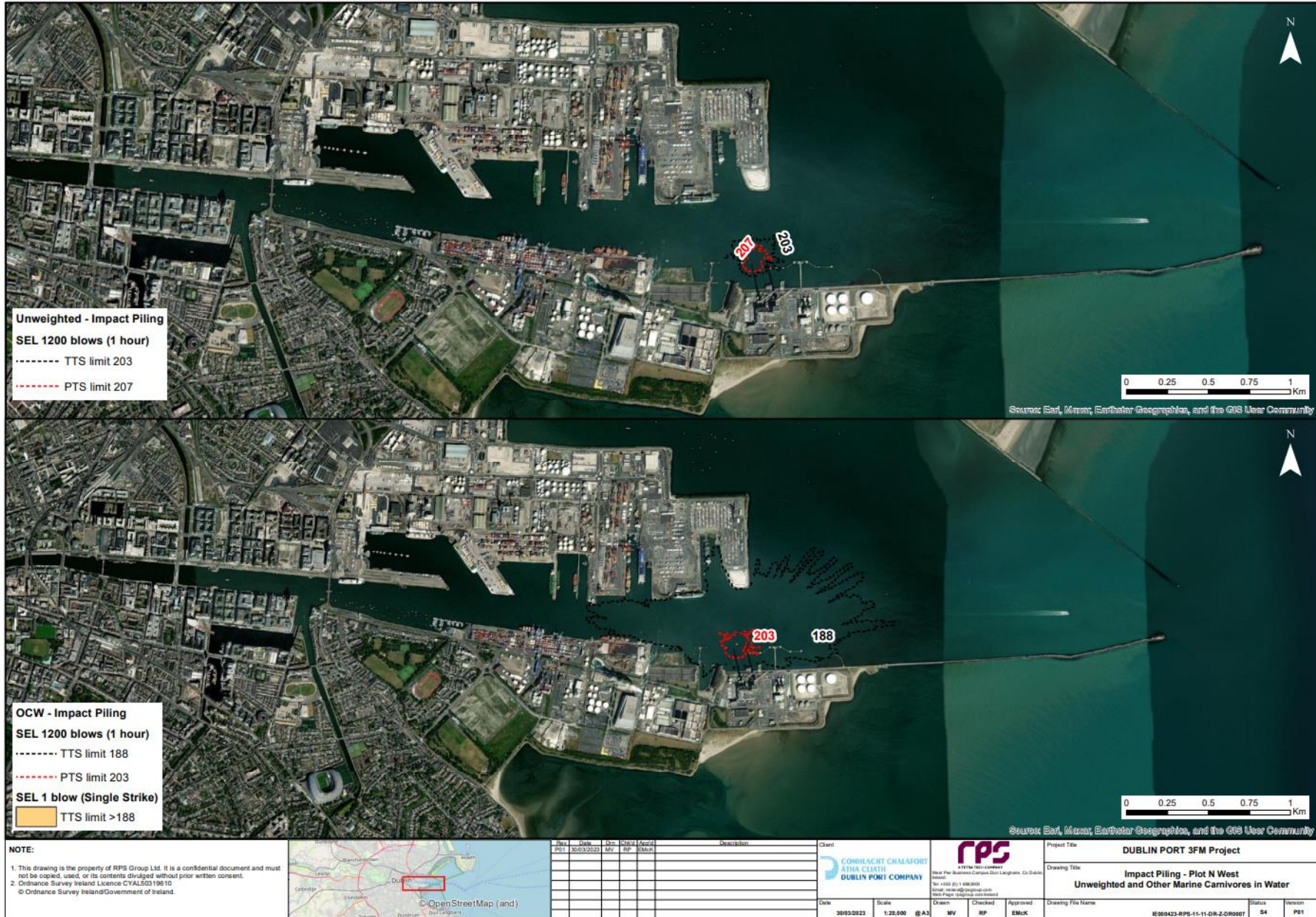
Figure 12.2.20. Impact piling, Area N west, Single piling rig, Fish (unweighted) and OCW hearing group.
