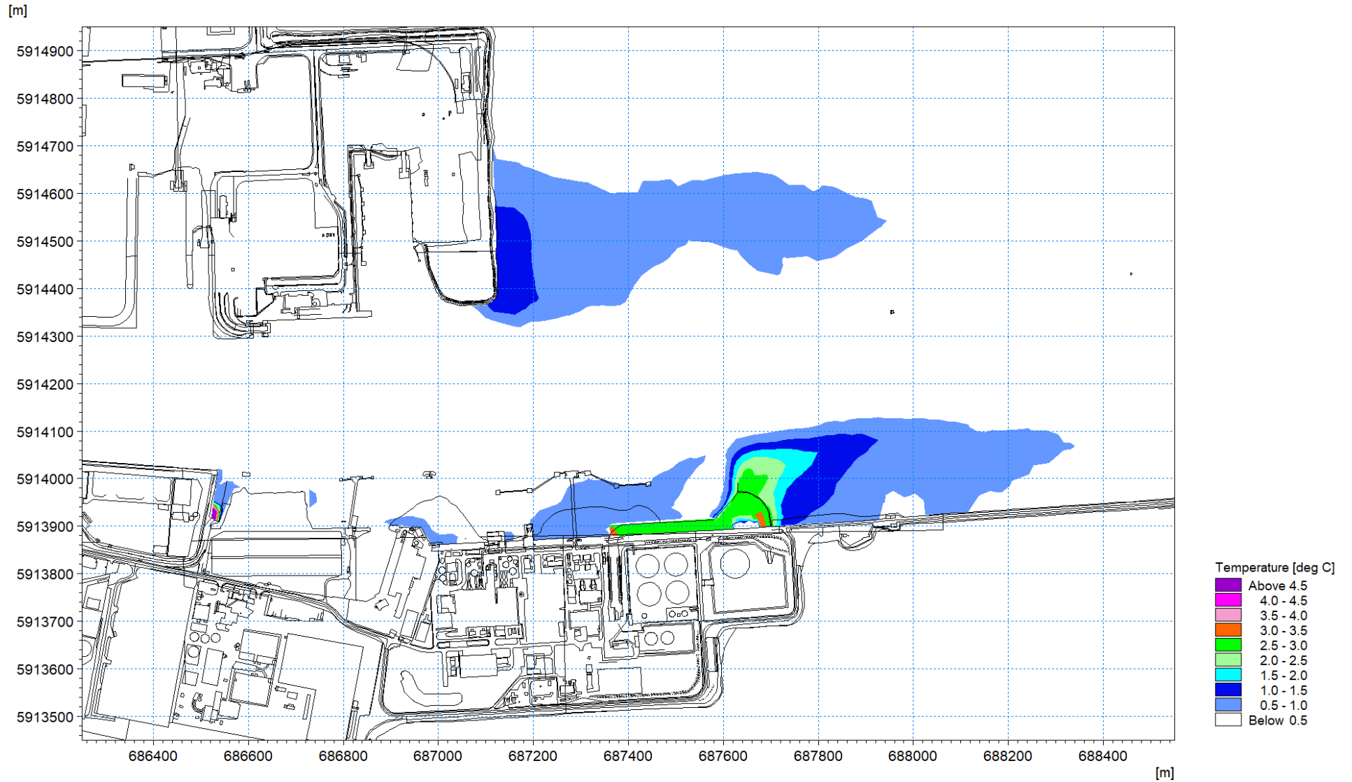
Figure 1.120: Thermal plume 9 th April 2019 – excess temperature at high water circa 0.9m depth layer 5
