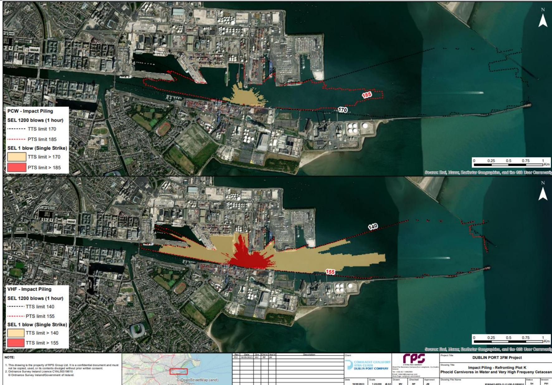
Figure 12.2.19. Impact piling, Area K, VHF and PCW hearing group.
