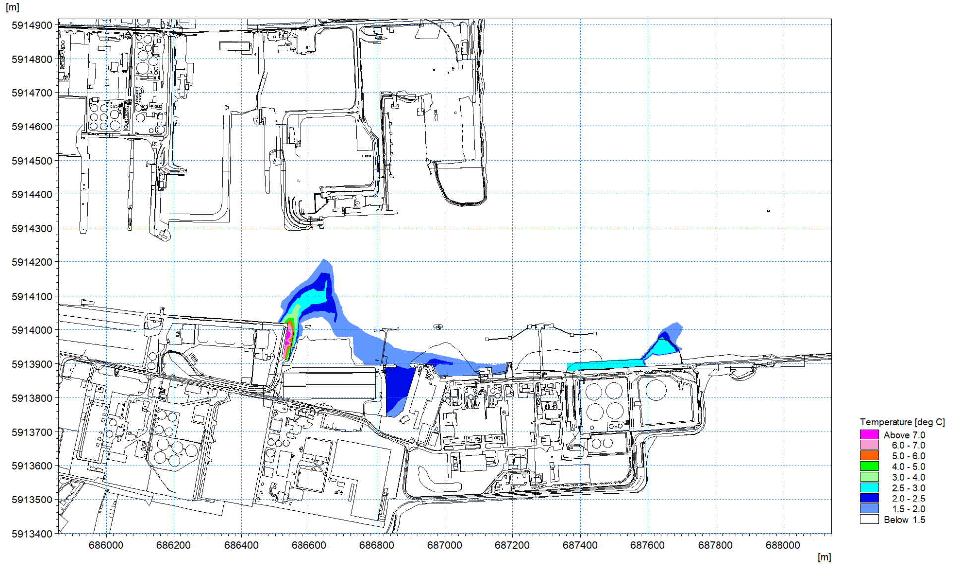
Figure 1.83: Thermal plume 20 th April 2018 – excess temperature at mid-flood circa 1m depth layer 5
