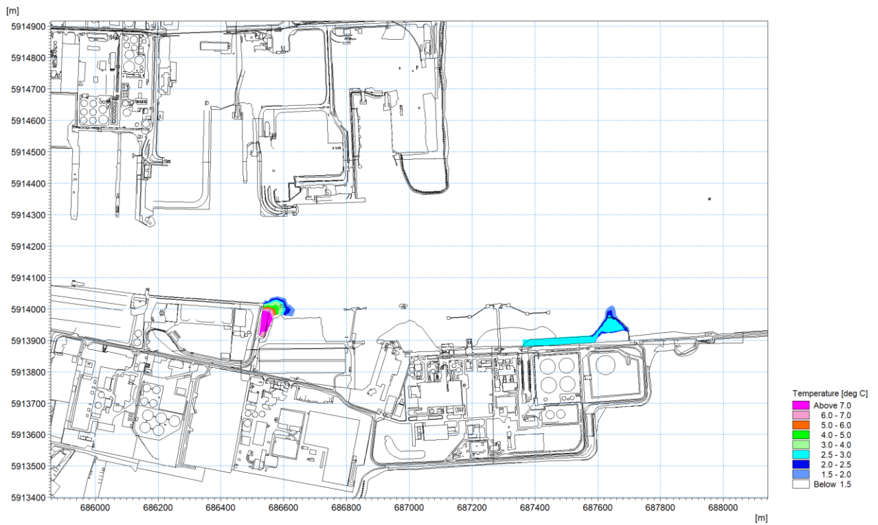
Figure 1.20: Thermal plume 20 th April 2018 – excess temperature at mid-flood circa 1m depth.
