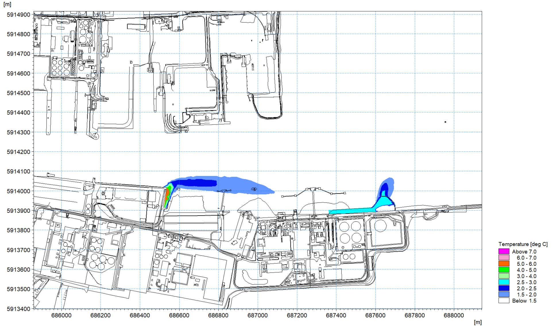
Figure 1.79: Thermal plume 12 th August 2016 – excess temperature at mid-flood circa 0.3m depth layer 6
