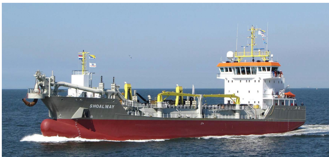
Figure 2.1: The trailing suction hopper dredger “Shoalway” used for the March 2020 capital dredging campaign within the inner Liffey channel
