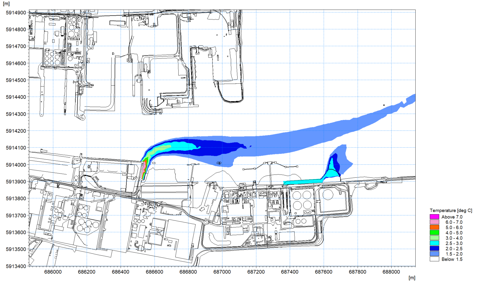
Figure 1.100: Thermal plume 24 th April 2018 – excess temperature at mid-ebb circa 0.3m depth layer 6
