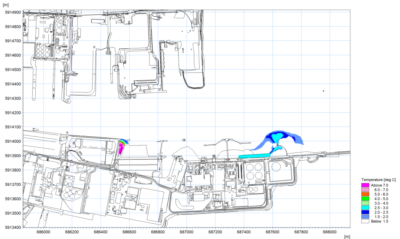
Figure 1.32: Thermal plume 20 th April 2018 – excess temperature at low water circa 1m depth.
