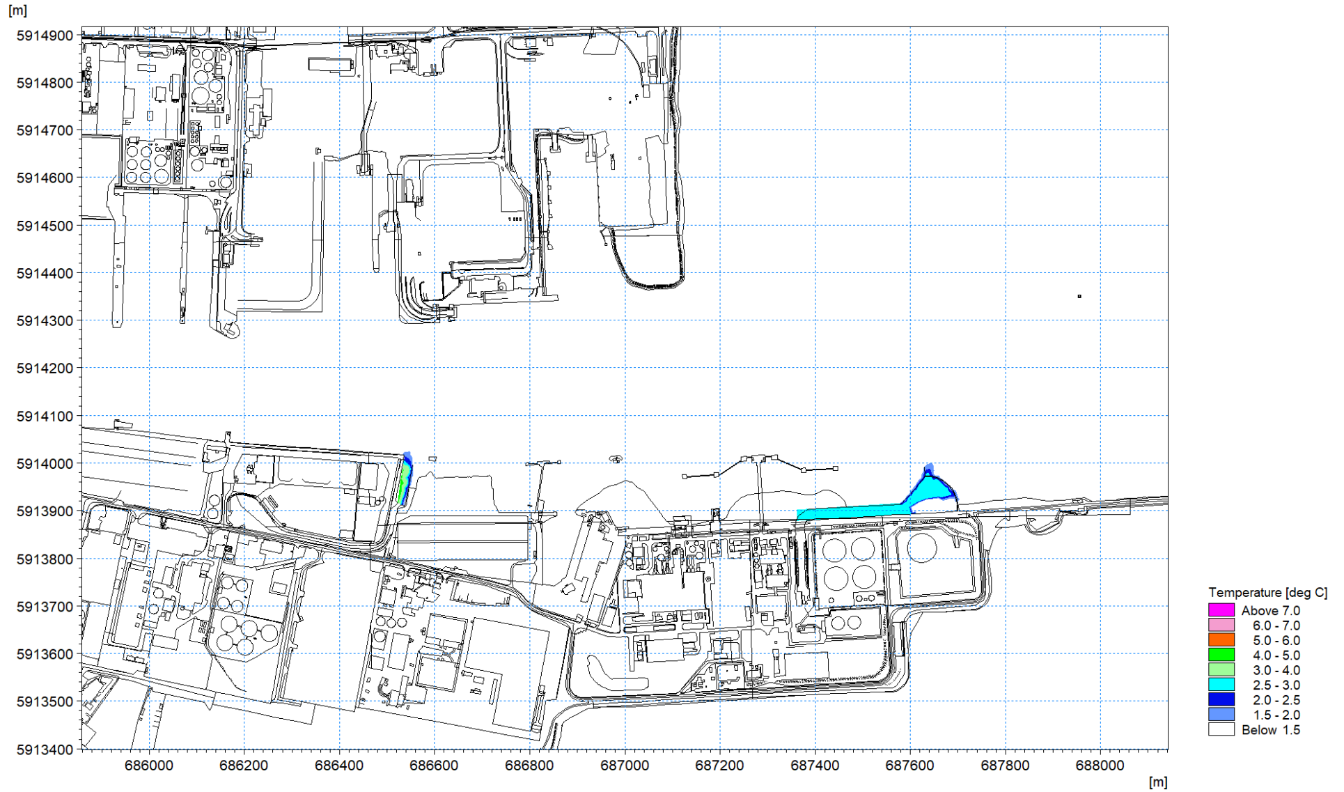
Figure 1.72: Thermal plume 12 th August 2016 – excess temperature at high water circa 2m depth layer 4
