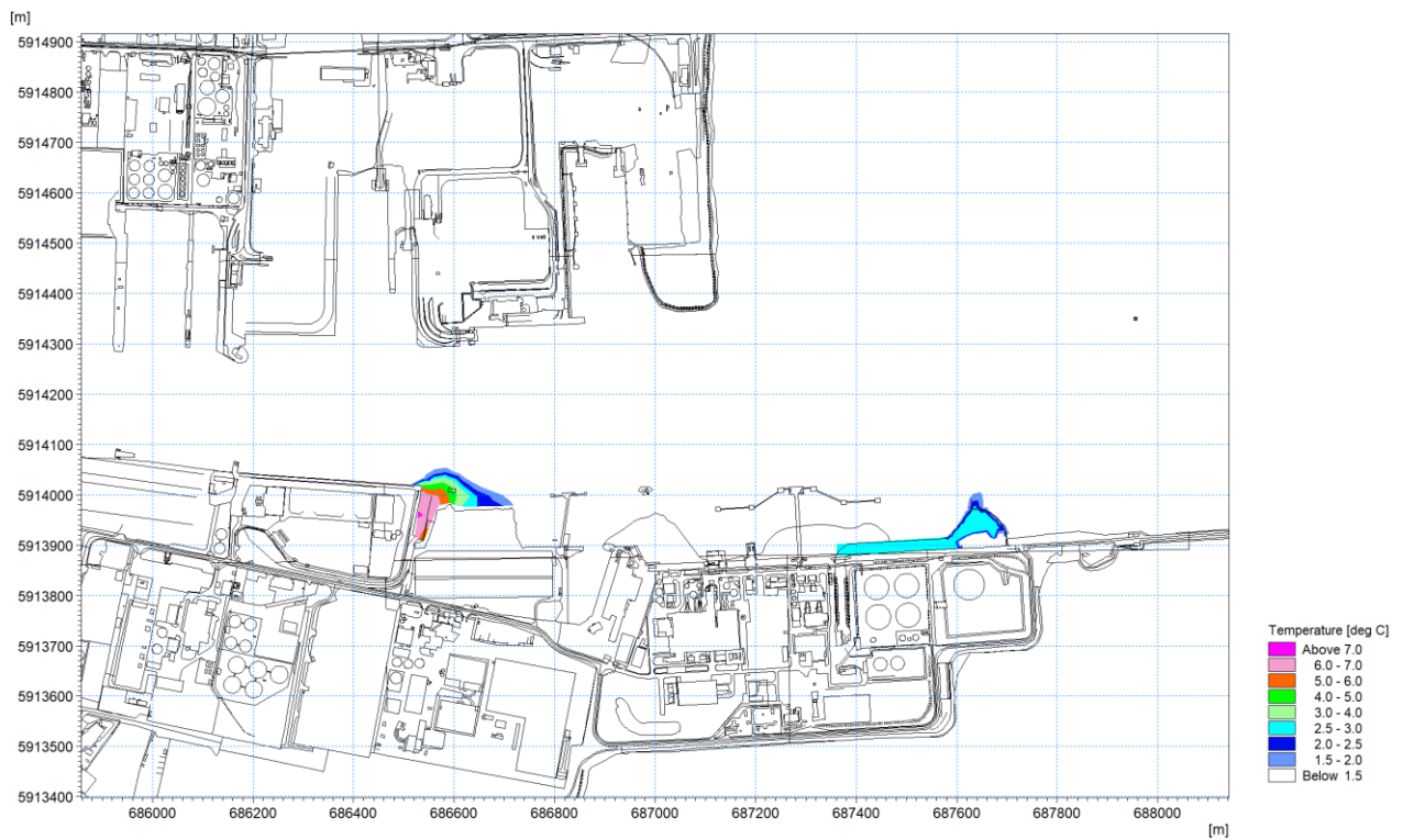
Figure 1.28: Thermal plume 20 th April 2018 – excess temperature at mid-ebb circa 1m depth.
