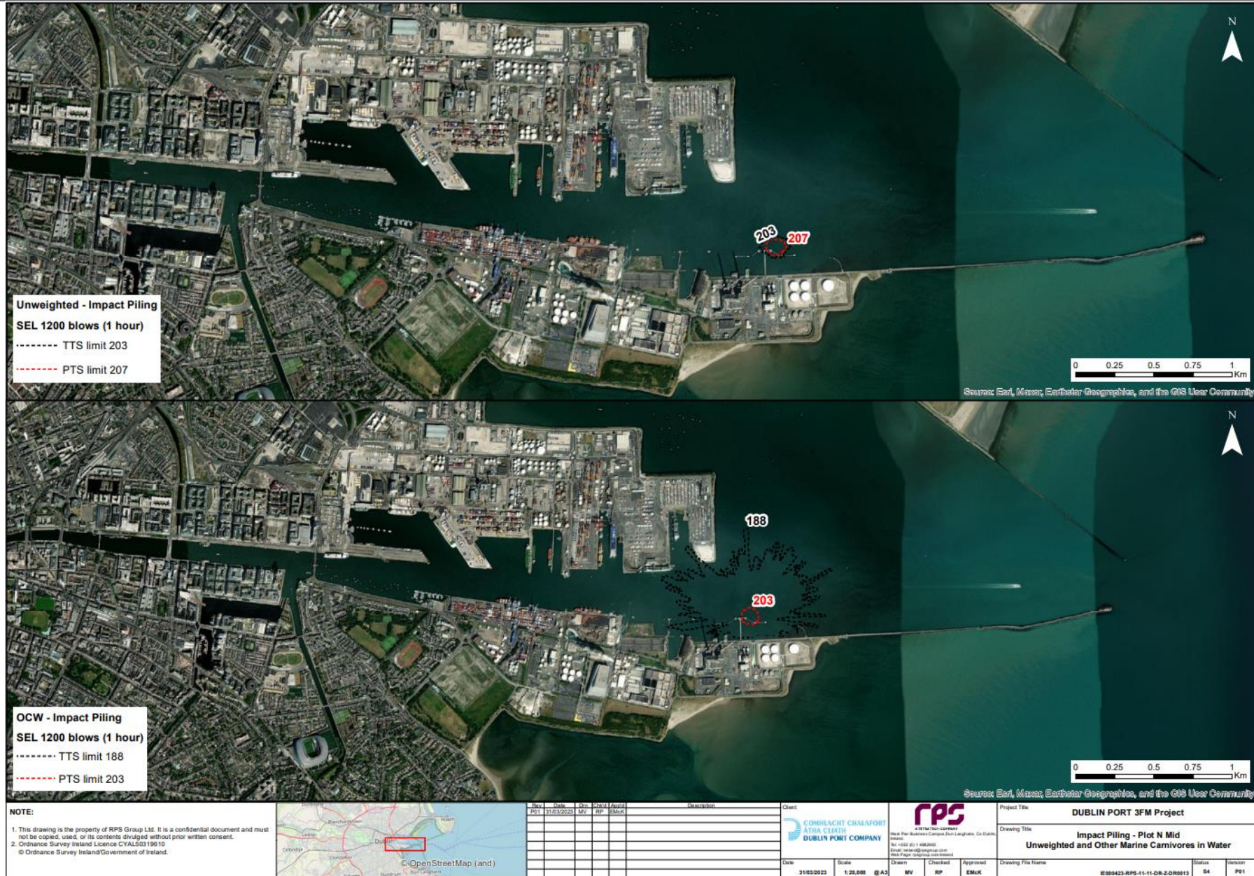
Figure 12.2.22. Impact piling, Area N middle, Single piling rig, Fish (unweighted) and OCW hearing group.
