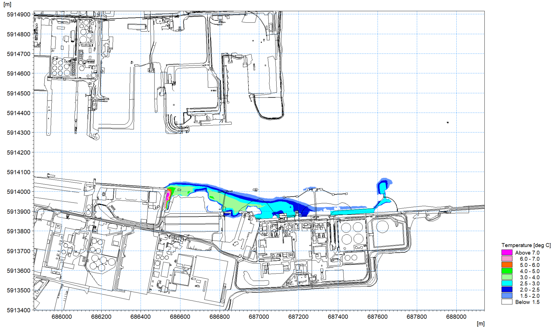
Figure 1.93: Thermal plume 20 th April 2018 – excess temperature at low water circa 2m depth layer 4
