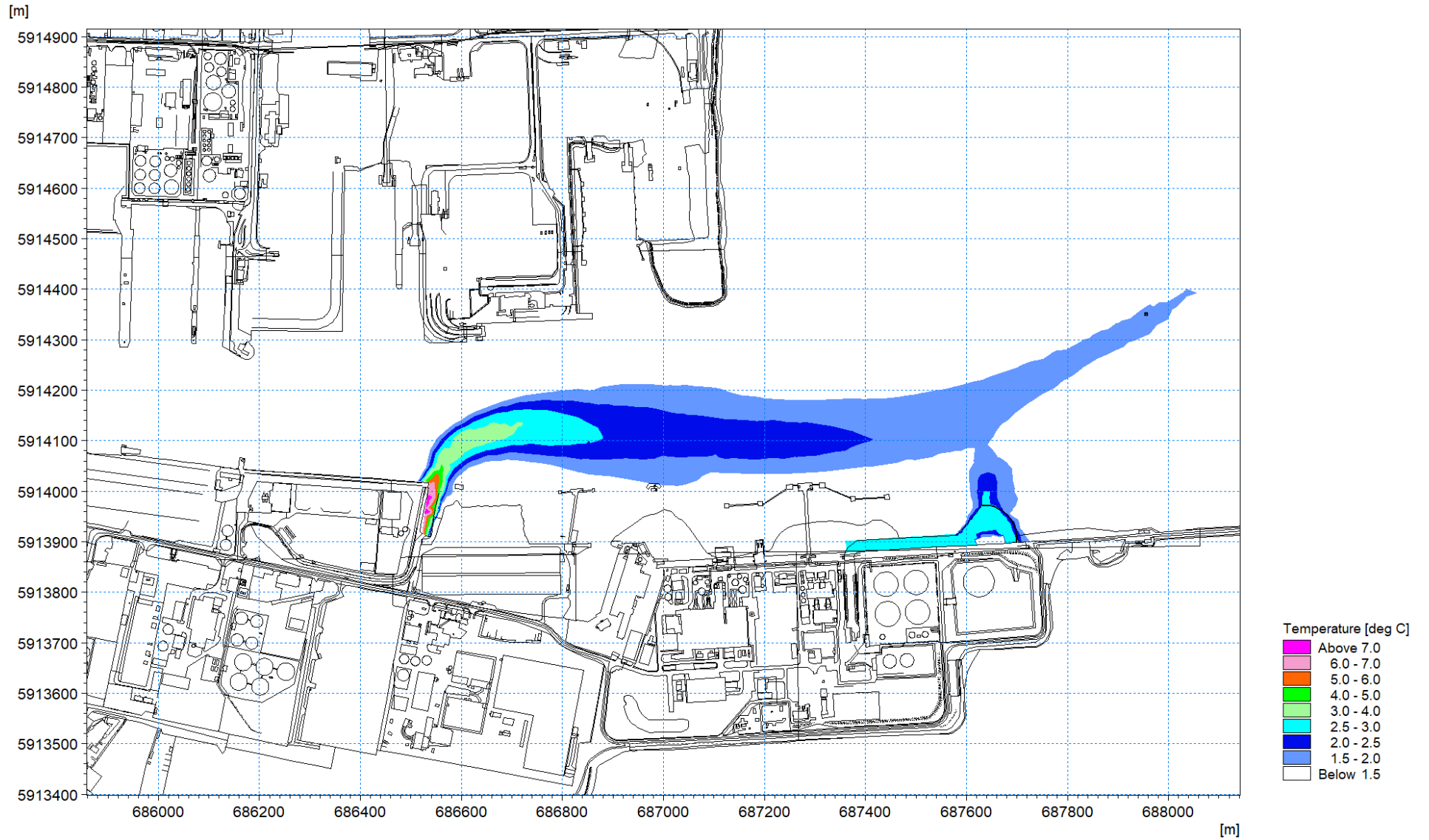
Figure 1.97: Thermal plume 24 th April 2018 – excess temperature at high water circa 0.3m depth layer 6
