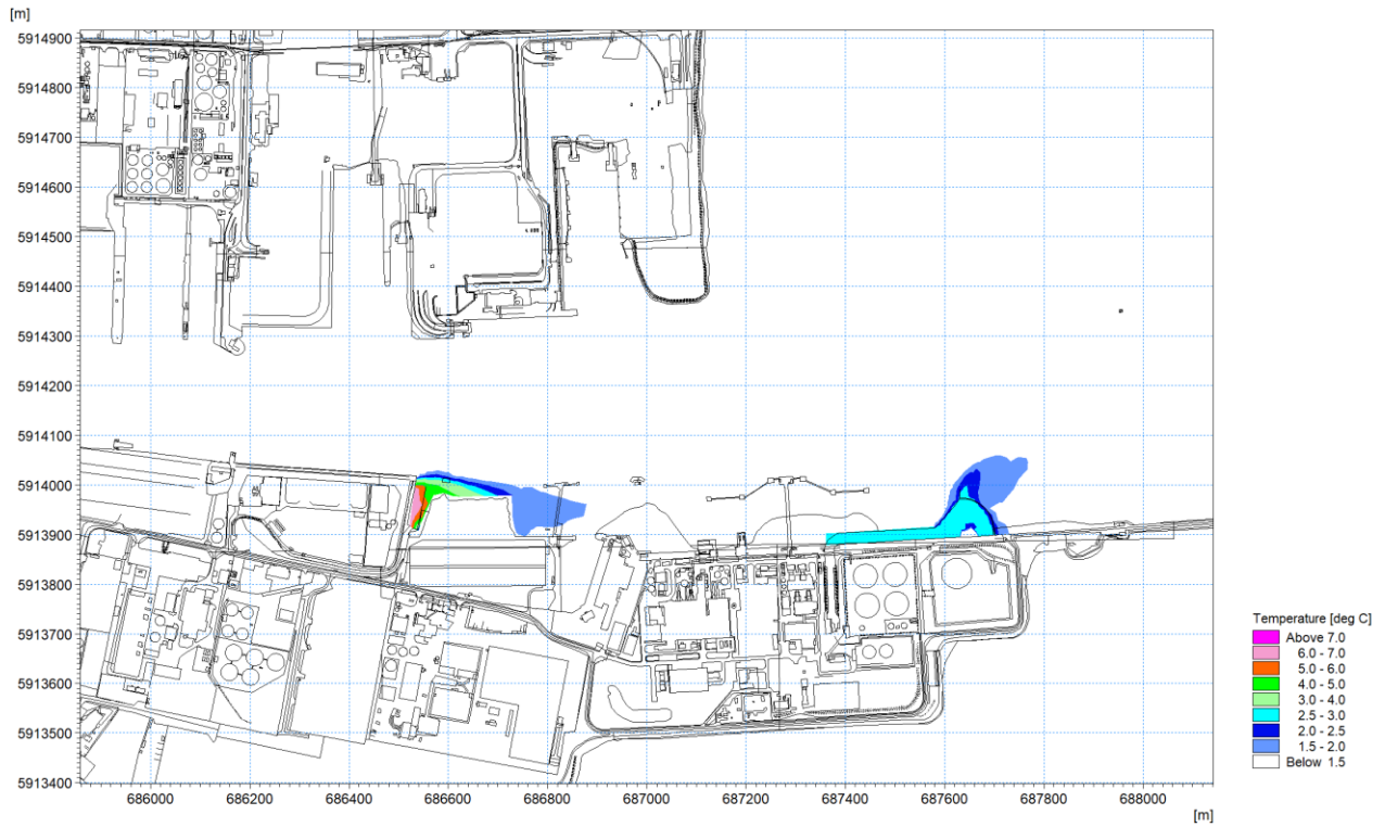
Figure 1.23: Thermal plume 20 th April 2018 – excess temperature at high water circa 0.3m depth.
