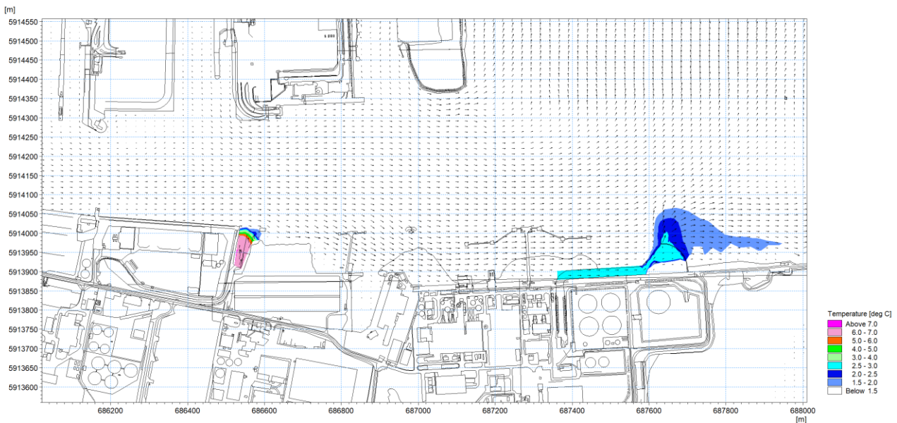
Figure 1.38: Thermal plume 24 th April 2018 – excess temperature at mid-flood circa 0.3m depth.
