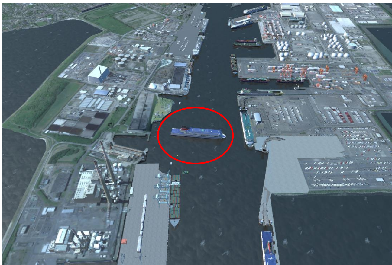
Figure 24 Example visual scene from HR Wallingford's Ship Simulator, illustrating the Turning Circle in use. Turning Circle shown indicatively in red. View looking west.
