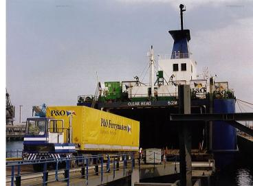
Freight units are typically 13.6 metre long trailers of varying types including refrigerated units, curtain-sided trailers, flat trailers and car transporters. There are also smaller freight units including non-articulated trucks and vans.
