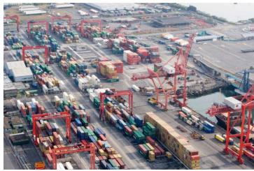
Secondary handling equipment refers to the equipment (usually gantry cranes of one type or another) used to store containers in back areas in large stacks.
