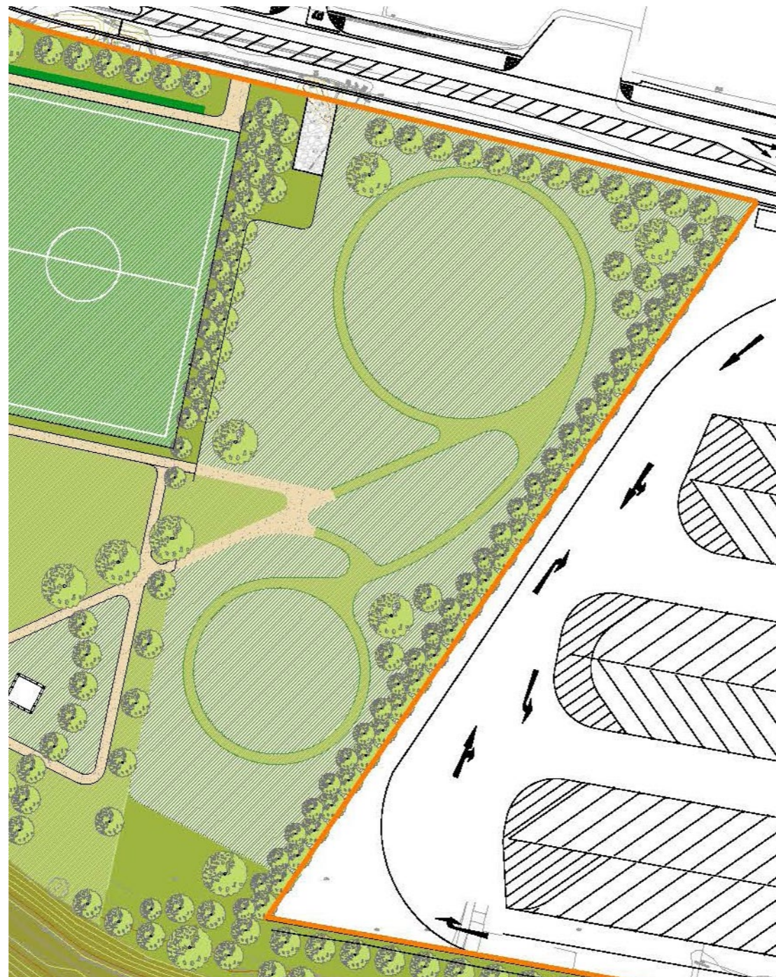
Configuration of wildflower meadow zone east of Sports grounds and open parkland, with mown pathways and all soft landscape proposals
