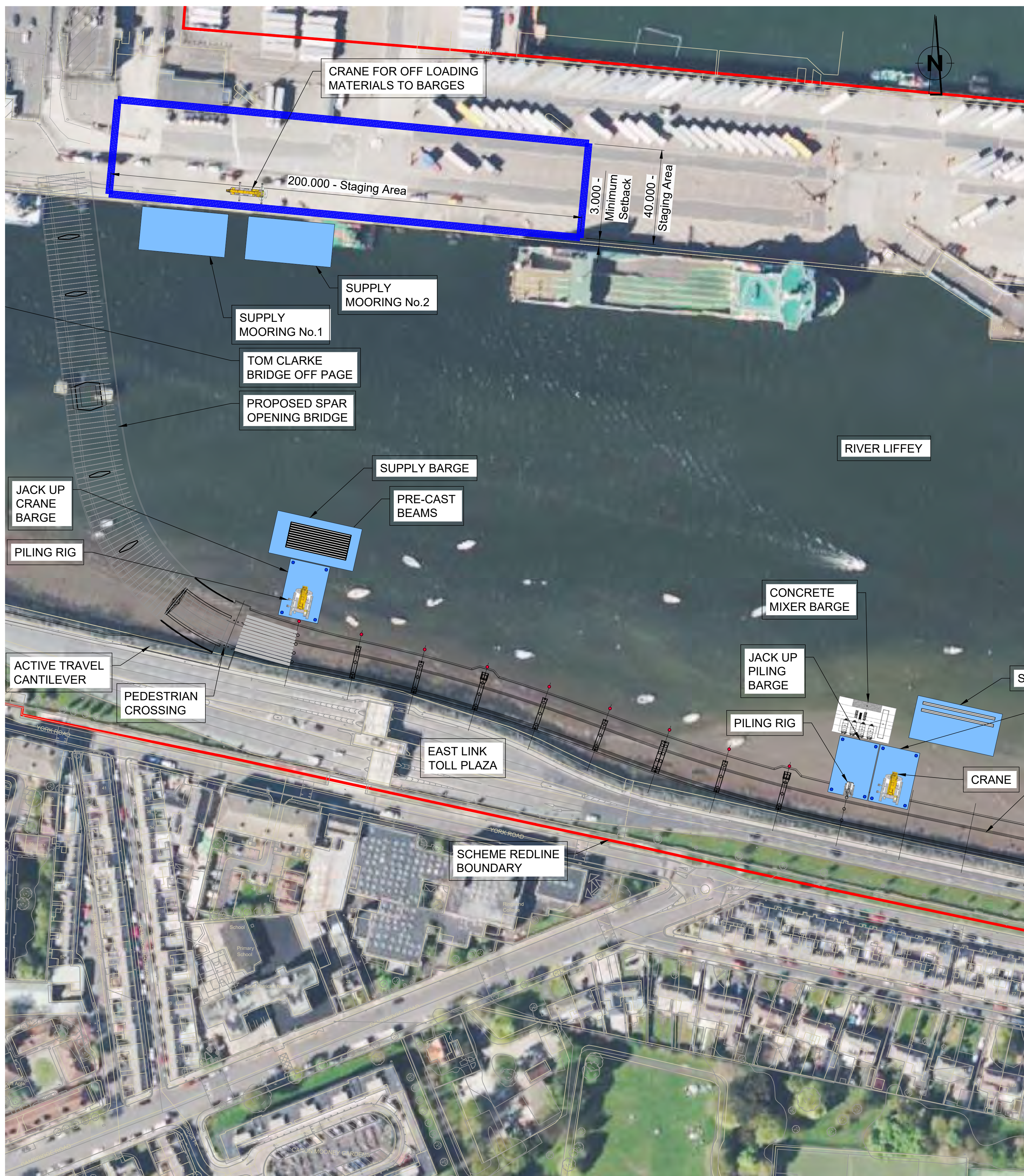
STAGE 7 - INSTALLATION OF PRE-CAST BEAMS AND PERMANENT FORMWORK - PLAN (Scale 1 : 1,000)
