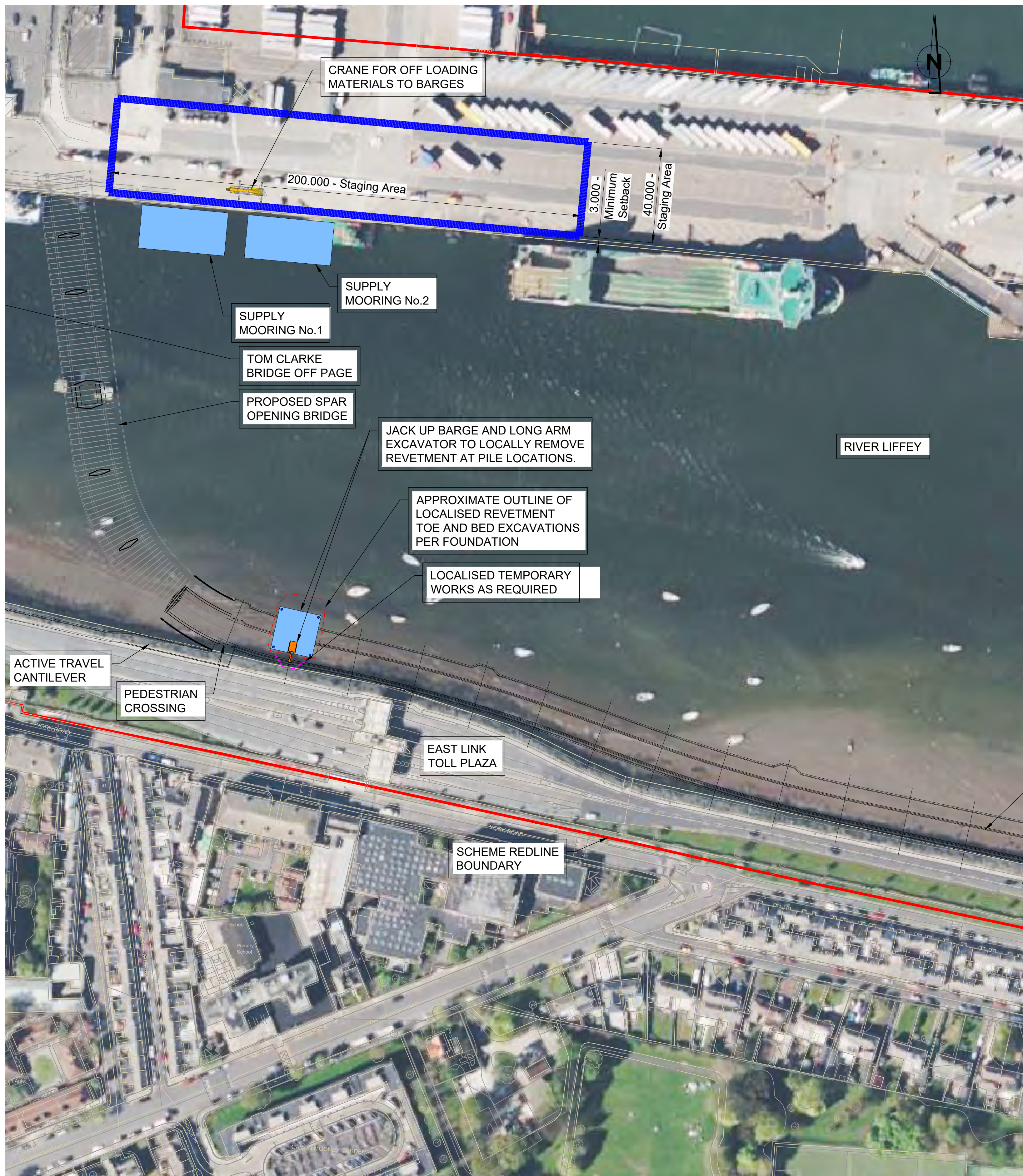
STAGE 2 - LOCALISED EXCAVATIONS AND ENABLING WORKS AT REVETMENT TOE - PLAN (Scale 1 : 1,000)
